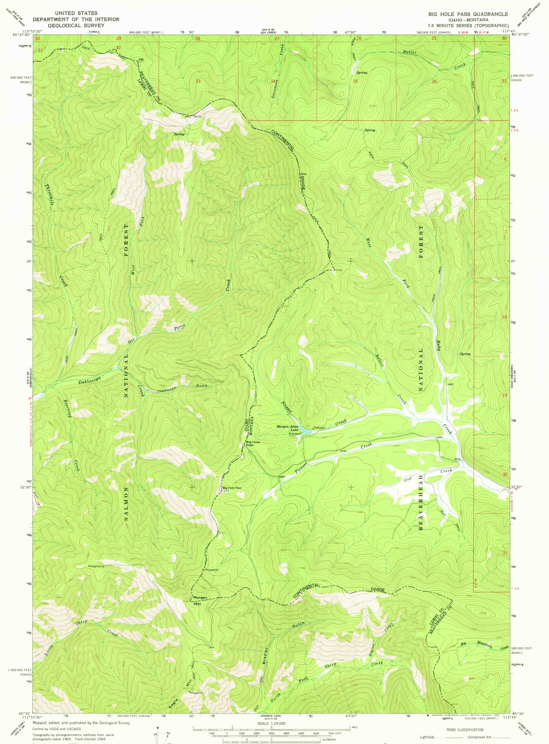
Polyconic projection. 1927 North American datum 10,000-foot grids based on Idaho coordinate system, central zone and Montana coordinate system, south zone 1000-meter Universal Transverse Mercator grid ticks, UTM GRID AND 1966 MAGNETIC NORTH DECLINATION AT CENTER OF SHEET zone 12, shown in blue To place on the predicted North American Datum 1983, move the projection lines 12 meters north and 70 meters east as shown by dashed corner ticks
