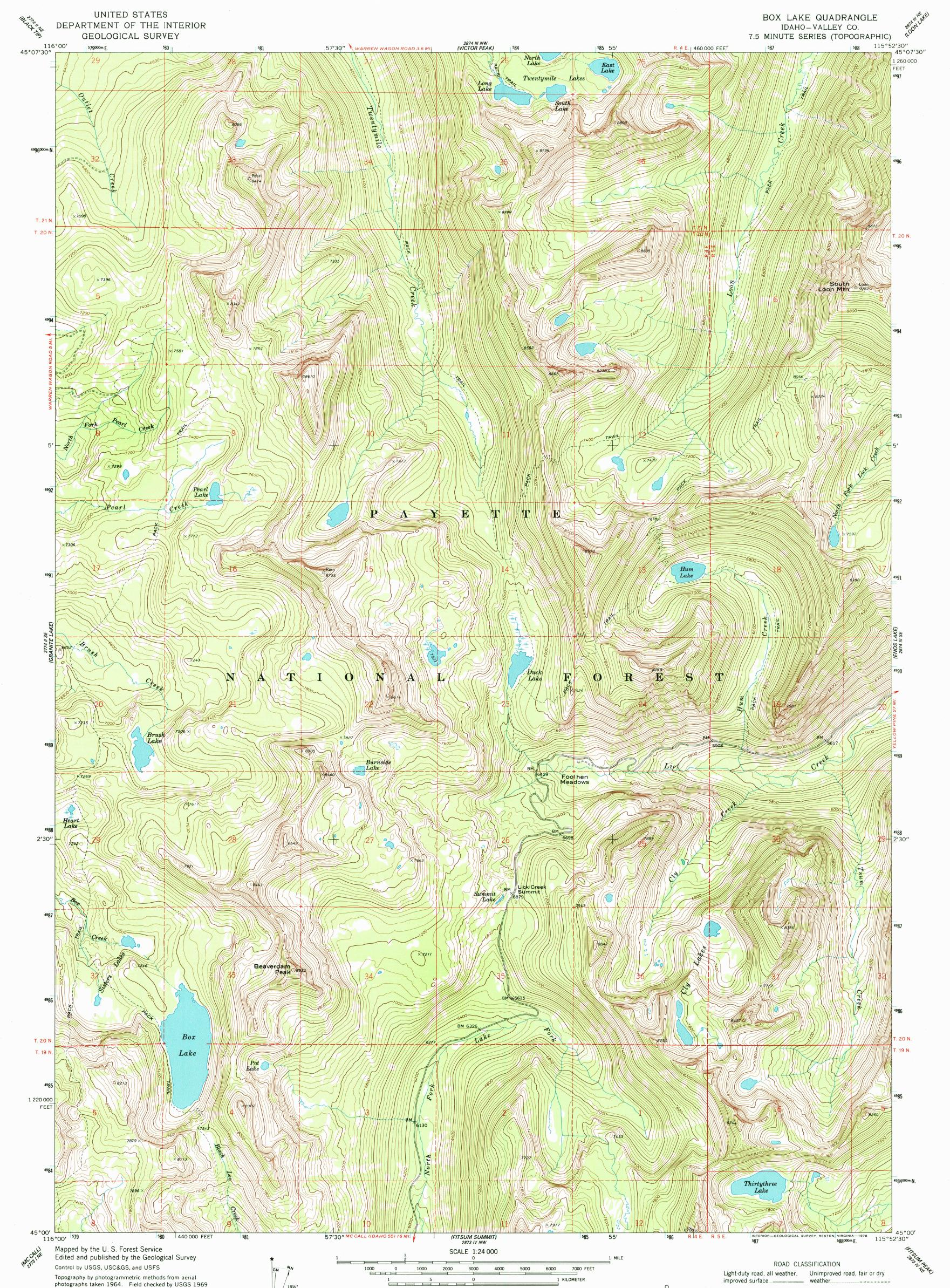
Polyconic projection. 1927 North American datum 10,000-foot grid based on Idaho coordinate system, west zone 1000-meter Universal Transverse Mercator grid ticks, zone 11, shown in blue UTM GRID AND 1969 MAGNETIC NORTH DECLINATION AT CENTER OF SHEET Where omitted, land lines have not been established
