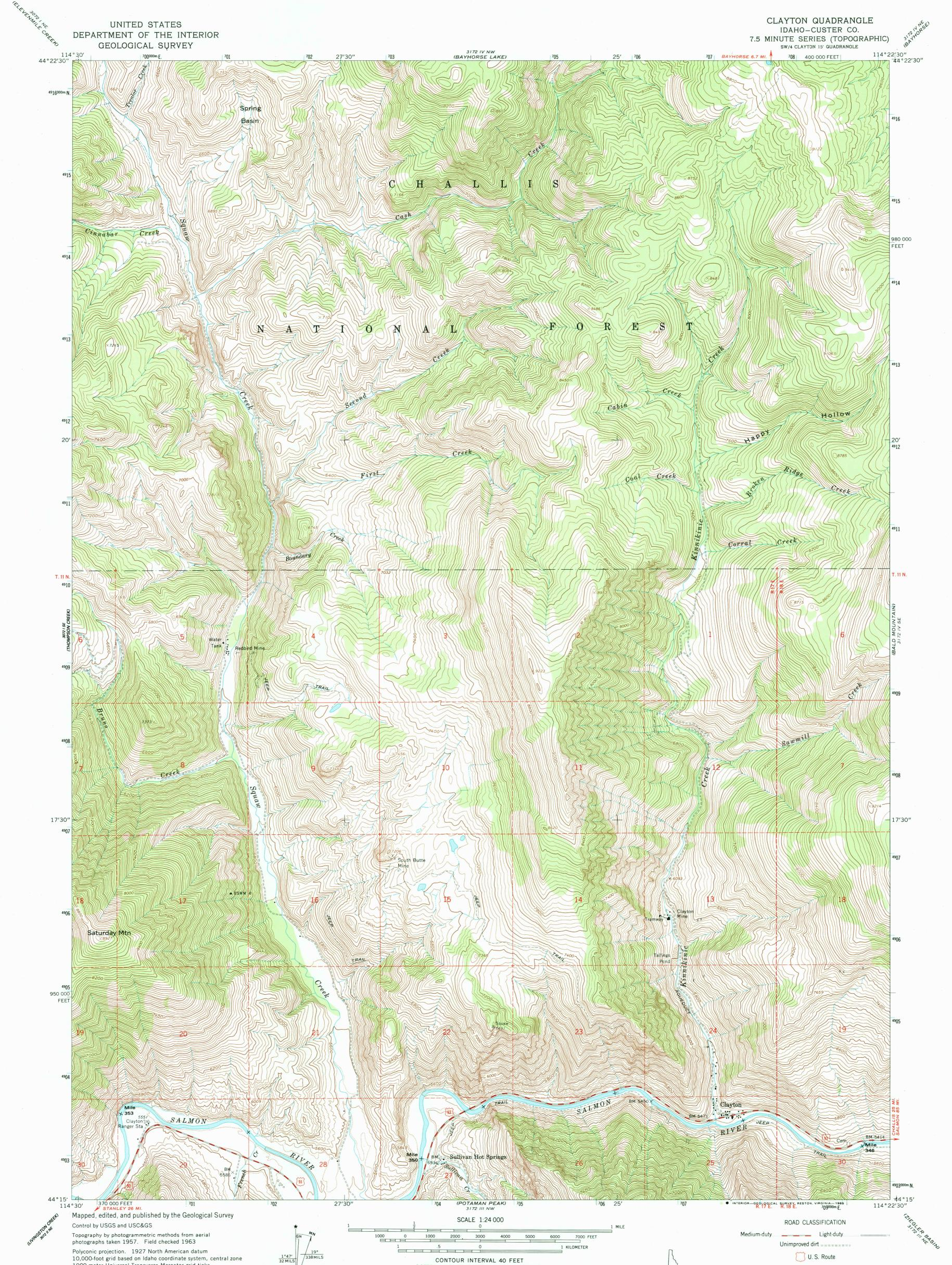
Polyconic projection. 1927 North American datum 10,000-foot grid based on Idaho coordinate system, central zone 1000-meter Universal Transverse Mercator grid ticks, zone 11, shown in blue To place on the predicted North American Datum 1983 move the projection lines 13 meters north and 72 meters east as shown by dashed corner ticks Where omitted, land lines have not been established There may be private inholdings within the boundaries of the National or State reservations shown on this map
