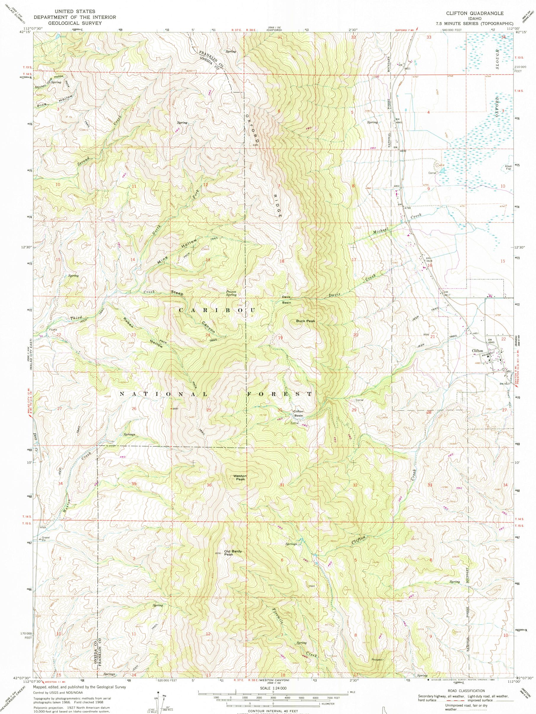
10,000-foot grid based on Idaho coordinate system, east zone 1000-meter Universal Transverse Mercator grid ticks, zone 12, shown in blue To place on the predicted North American Datum 1983, move the projection lines 12 meters north and 66 meters east as shown by dashed corner ticks
