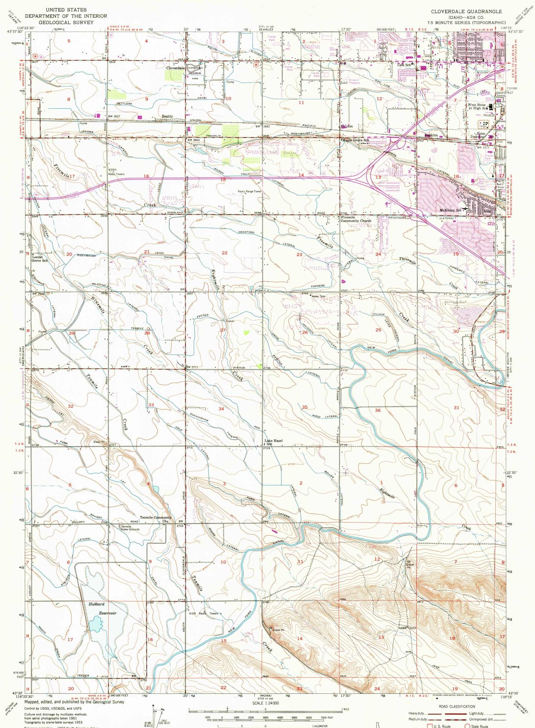
Topography by plane-table surveys 1953 Polyconic projection. 1927 North American datum 10,000-foot grid based on Idaho coordinate system, west zone 1000-meter Universal Transverse Mercator grid ticks, UTM GRID AND 1971 MAGNETIC NORTH DECLINATION AT CENTER OF SHEET zone 11, shown in blue
