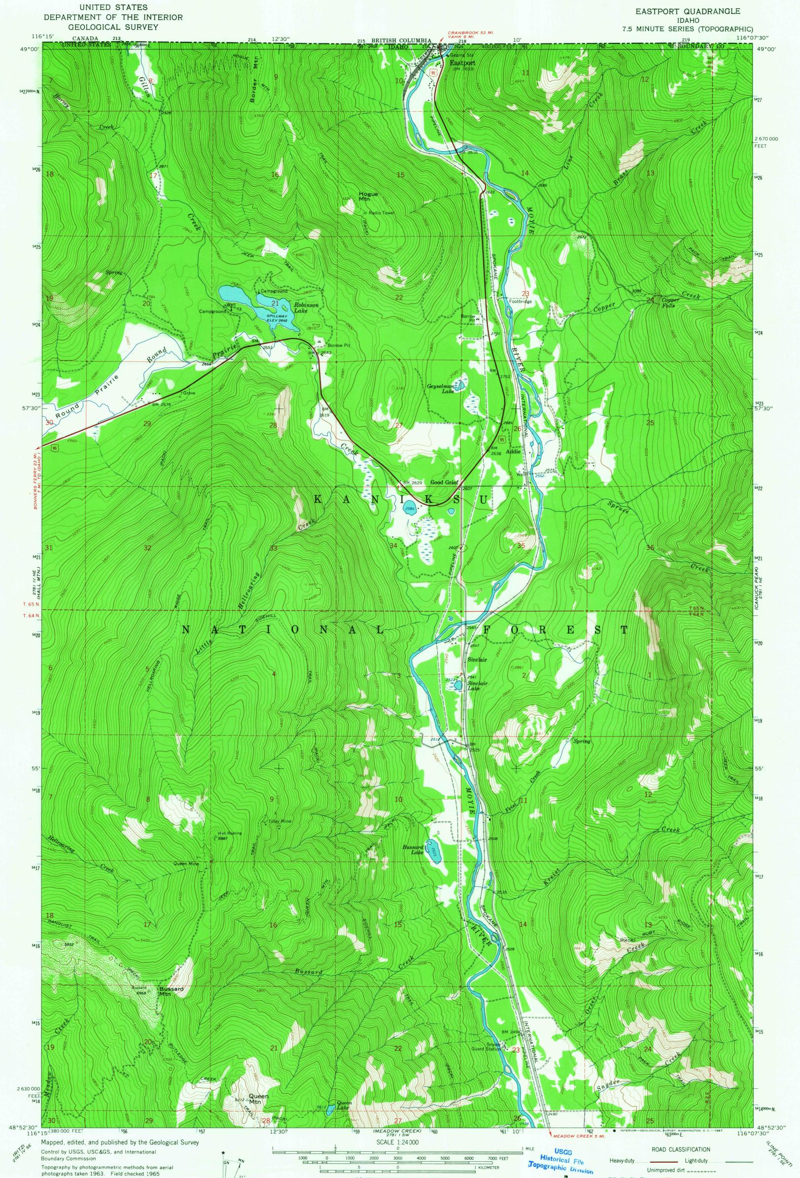
Polyconic projection. 1927 North American datum 10.000-foot grids based on Idaho coordinate system, west zone 1000-meter Universal Transverse Mercator grid ticks, zone 11, shown in blue Fine red dashed lines indicate selected fence lines Where omitted, land lines have not been established
