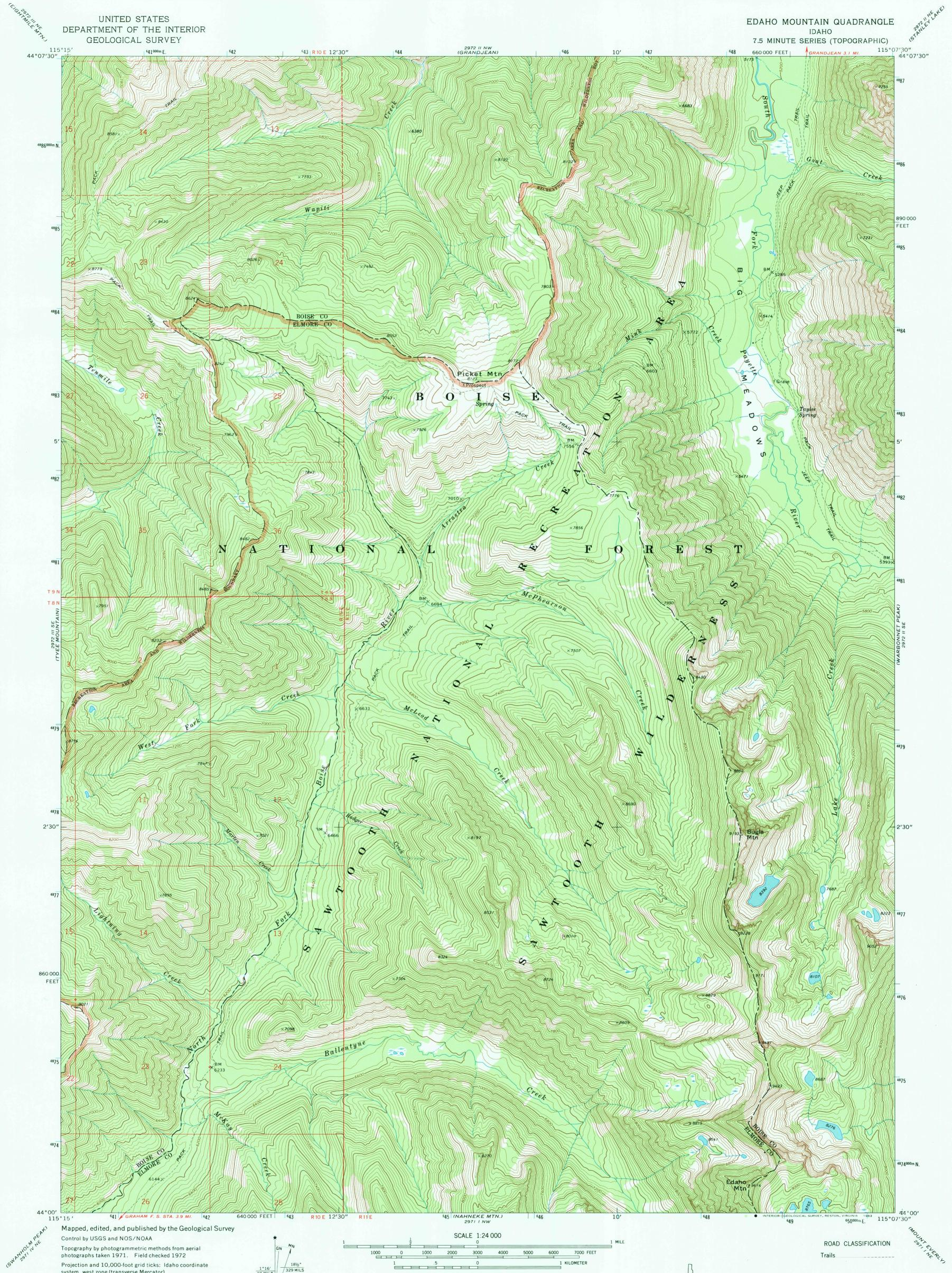
system, west zone (transverse Mercator) 1000-metre Universal Transverse Mercator grid ticks, zone 11, shown in blue. 1927 North American datum To place on the predicted North American Datum 1983 move the projection lines 14 meters north and 74 meters east as shown by dashed corner ticks Where omitted, land lines have not been established There may be private inholdings within the boundaries of the National or State reservations shown on this map
