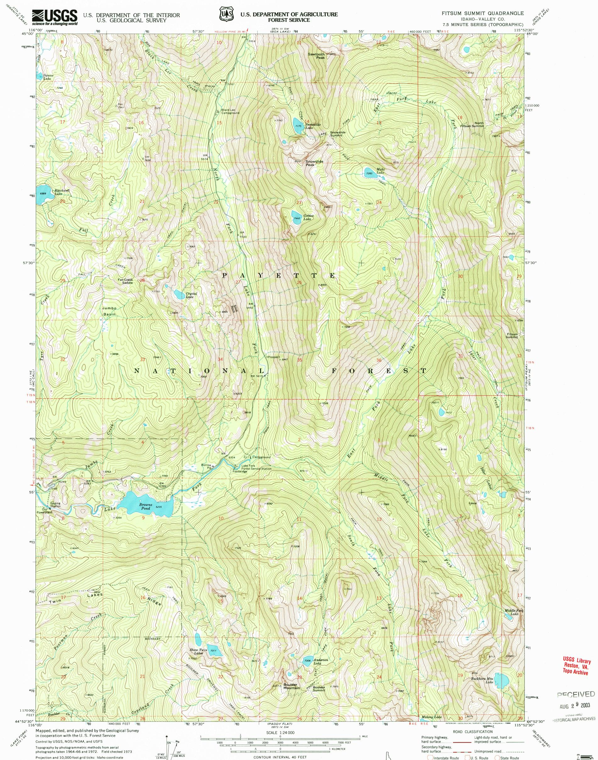
Projection and 10,000-foot grid ticks: Idaho coordinate system, west zone (transverse Mercator) 1000-meter Universal Transverse Mercator grid ticks, zone 11, shown in blue. 1927 North American datum To place on the predicted North American Datum 1983 move the projection lines 15 meters north and 76 meters east as shown by dashed corner ticks
