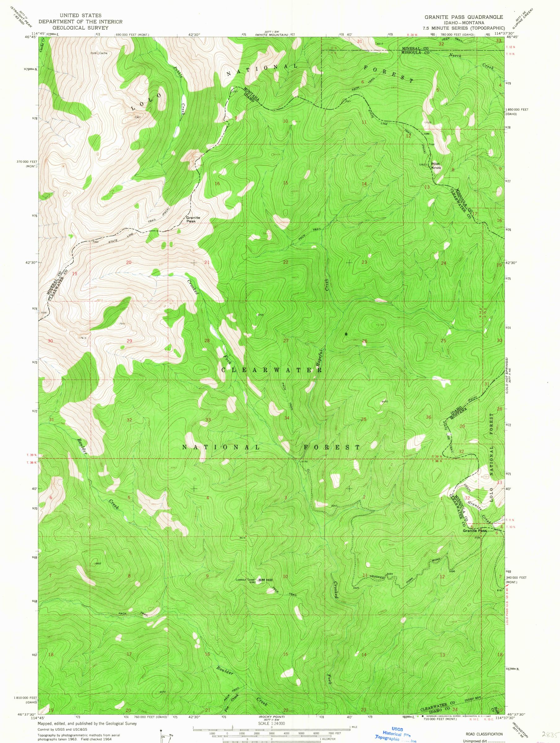
Polyconic projection. 1927 North American datum 1°41′ 30 MILS 10,000-foot grids based on Idaho coordinate system, west zone, and Montana coordinate system, central zone 1000-meter Universal Transverse Mercator grid ticks, zone 11, shown in blue UTM GRID AND 1964 MAGNETIC NORTH DECLINATION AT CENTER OF SHEET Where omitted, land lines have not been established
