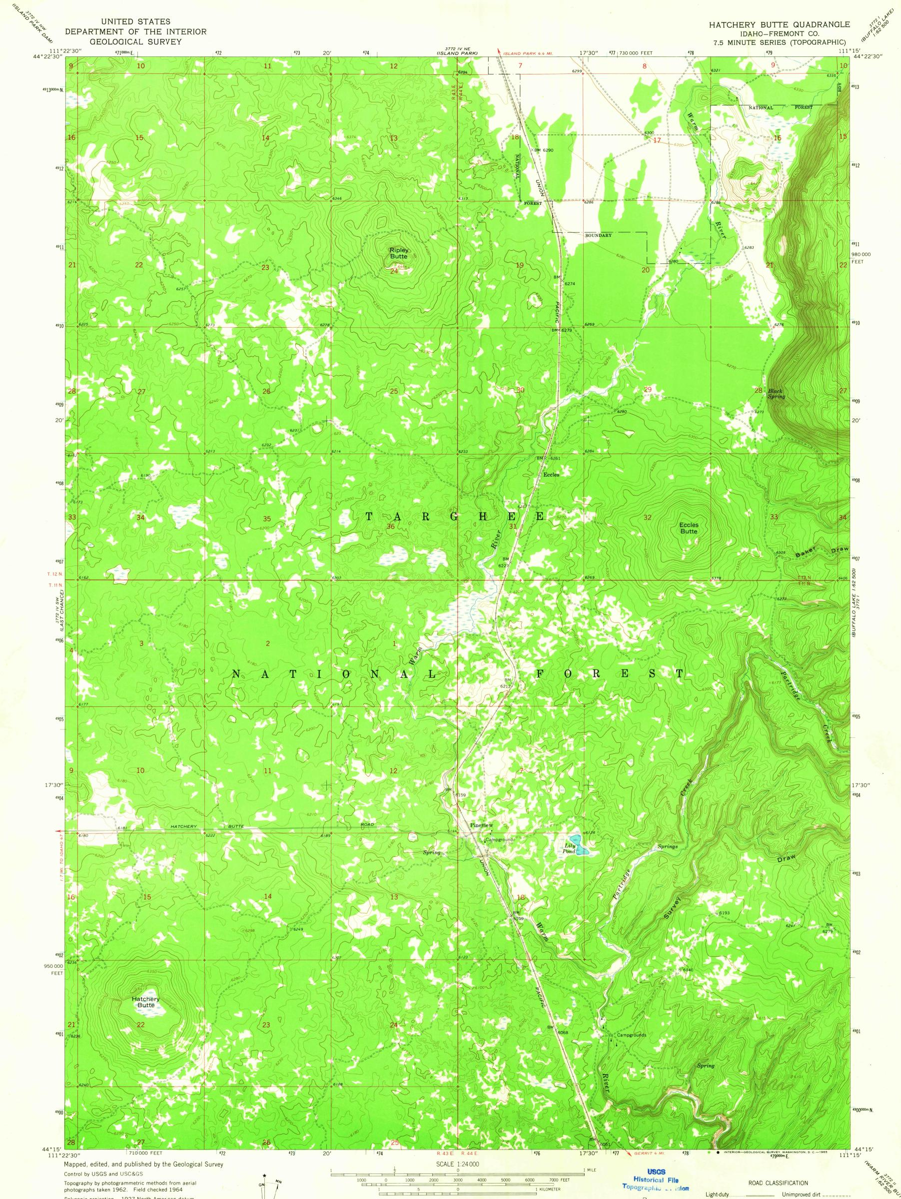
Polyconic projection. 1927 North American datum 10,000-foot grid based on Idaho coordinate system, east zone 1000-meter Universal Transverse Mercator grid ticks, zone 12, shown in blue UTM GRID AND 1964 MAGNETIC NORTH DECLINATION AT CENTER OF SHEET Where omitted, land lines have not been established
