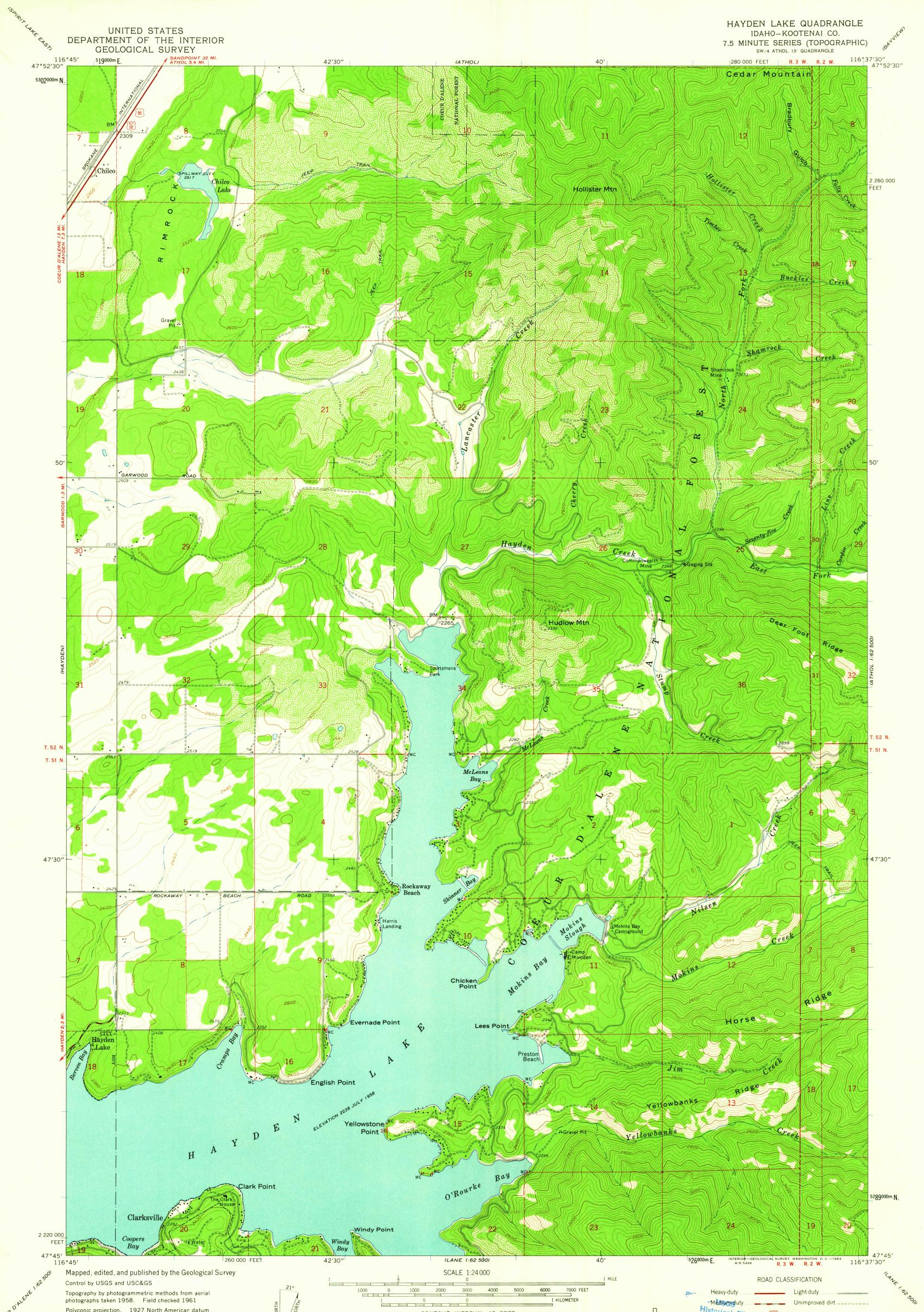
Polyconic projection. 1927 North American datum 10,000-foot grid based on Idaho coordinate system, west zone 1000-meter Universal Transverse Mercator grid ticks, zone 11, shown in blue
