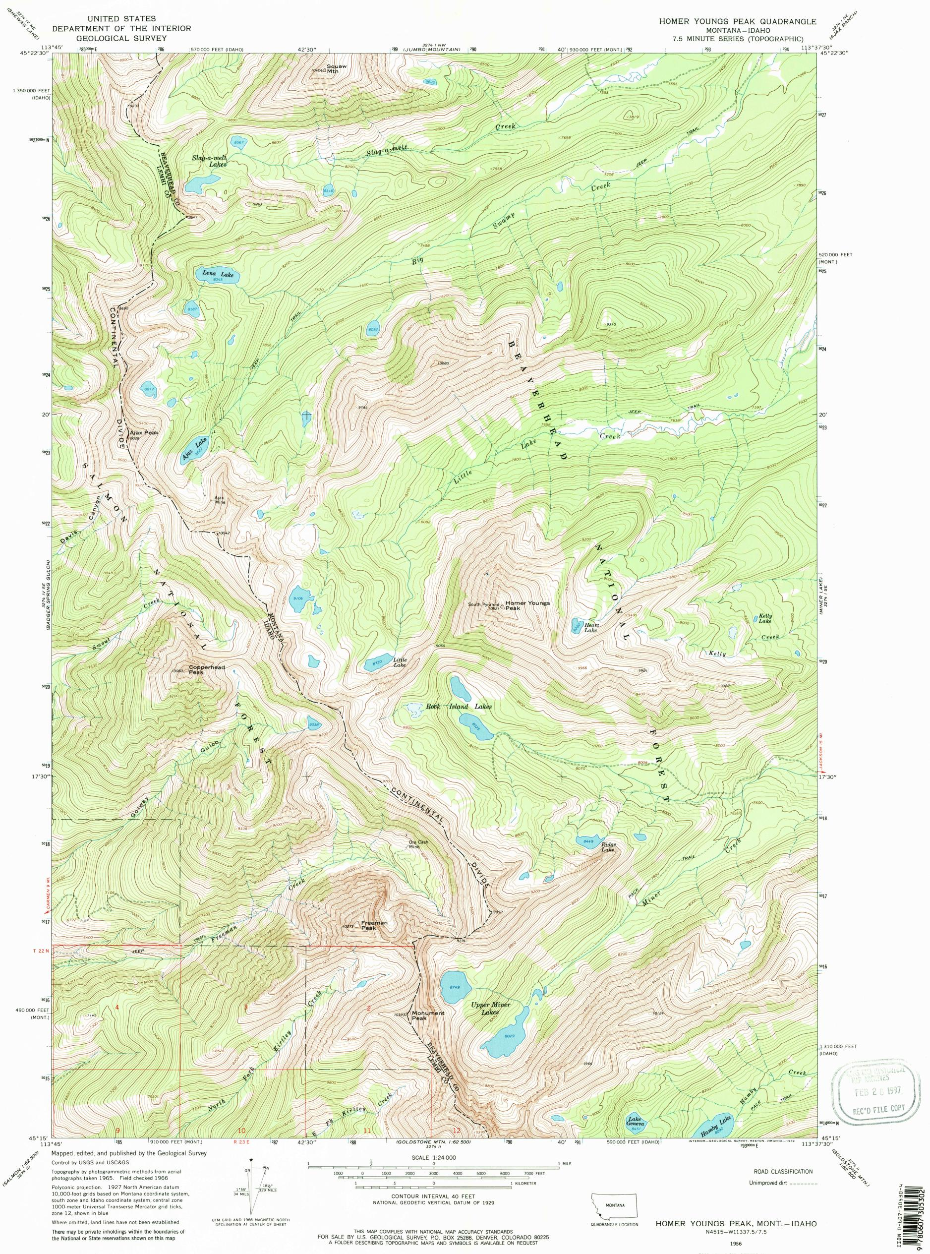
10,000-foot grids based on Montana coordinate system, south zone and Idaho coordinate system, central zone 1000-meter Universal Transverse Mercator grid ticks, zone 12, shown in blue
