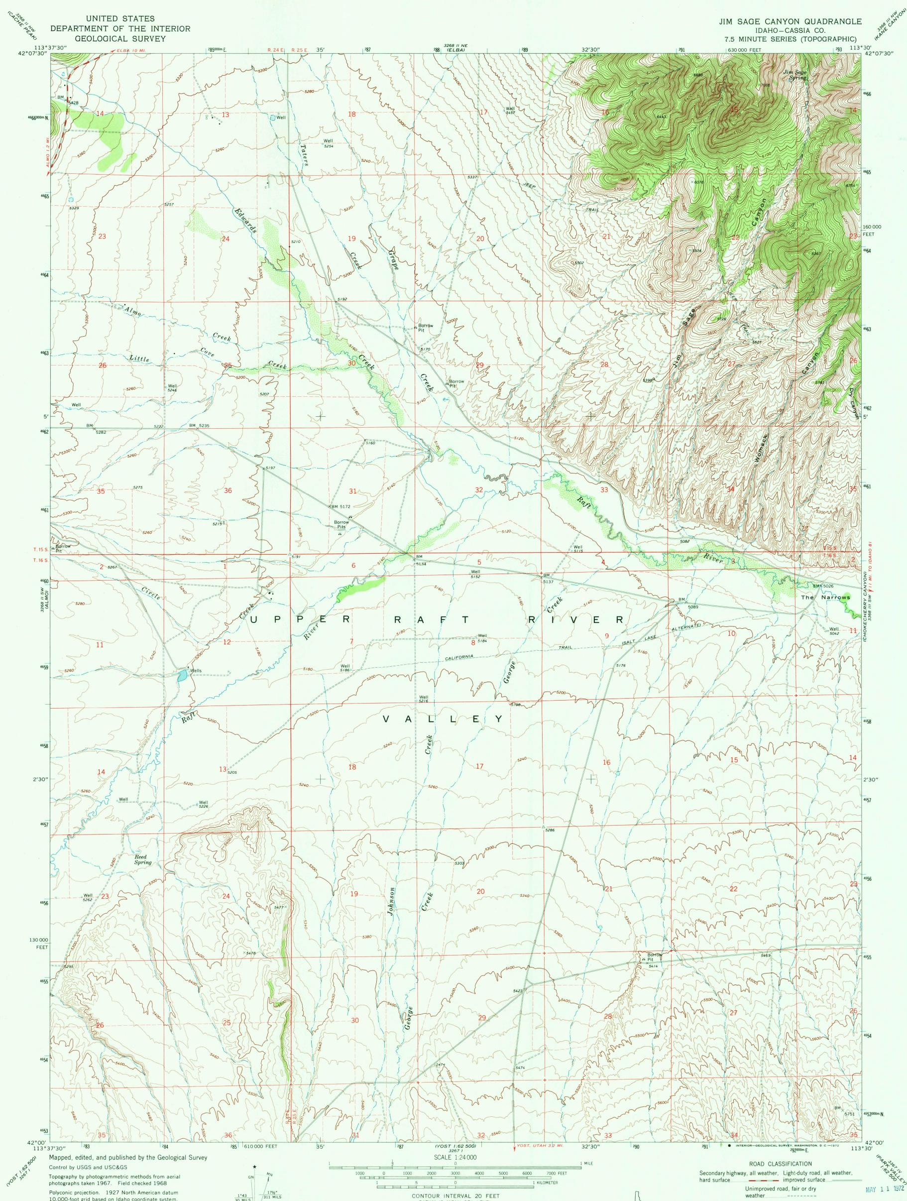
Polyconic projection. 1927 North American datum 10,000-foot grid based on Idaho coordinate system, central zone 1000-meter Universal Transverse Mercator grid ticks, zone 12, shown in blue
