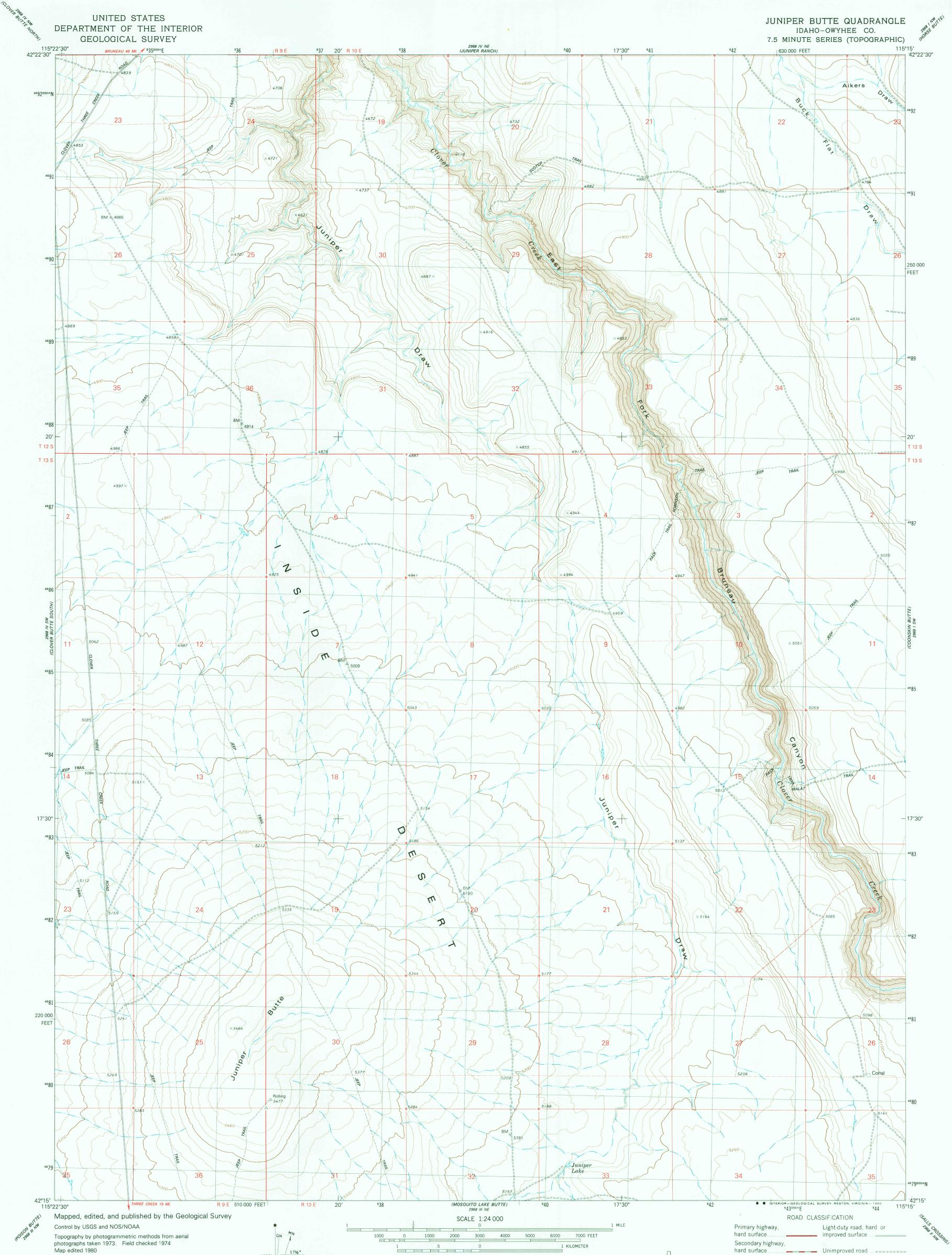
Projection and 10,000-foot grid ticks: Idaho coordinate system, west zone (transverse Mercator) 1000-meter Universal Transverse Mercator grid, zone 11 1927 North American Datum UTM GRID AND 1980 MAGNETIC NORTH DECLINATION AT CENTER OF SHEET To place on the predicted North American Datum 1983 move the projection lines 14 meters north and 75 meters east as shown by dashed corner ticks
