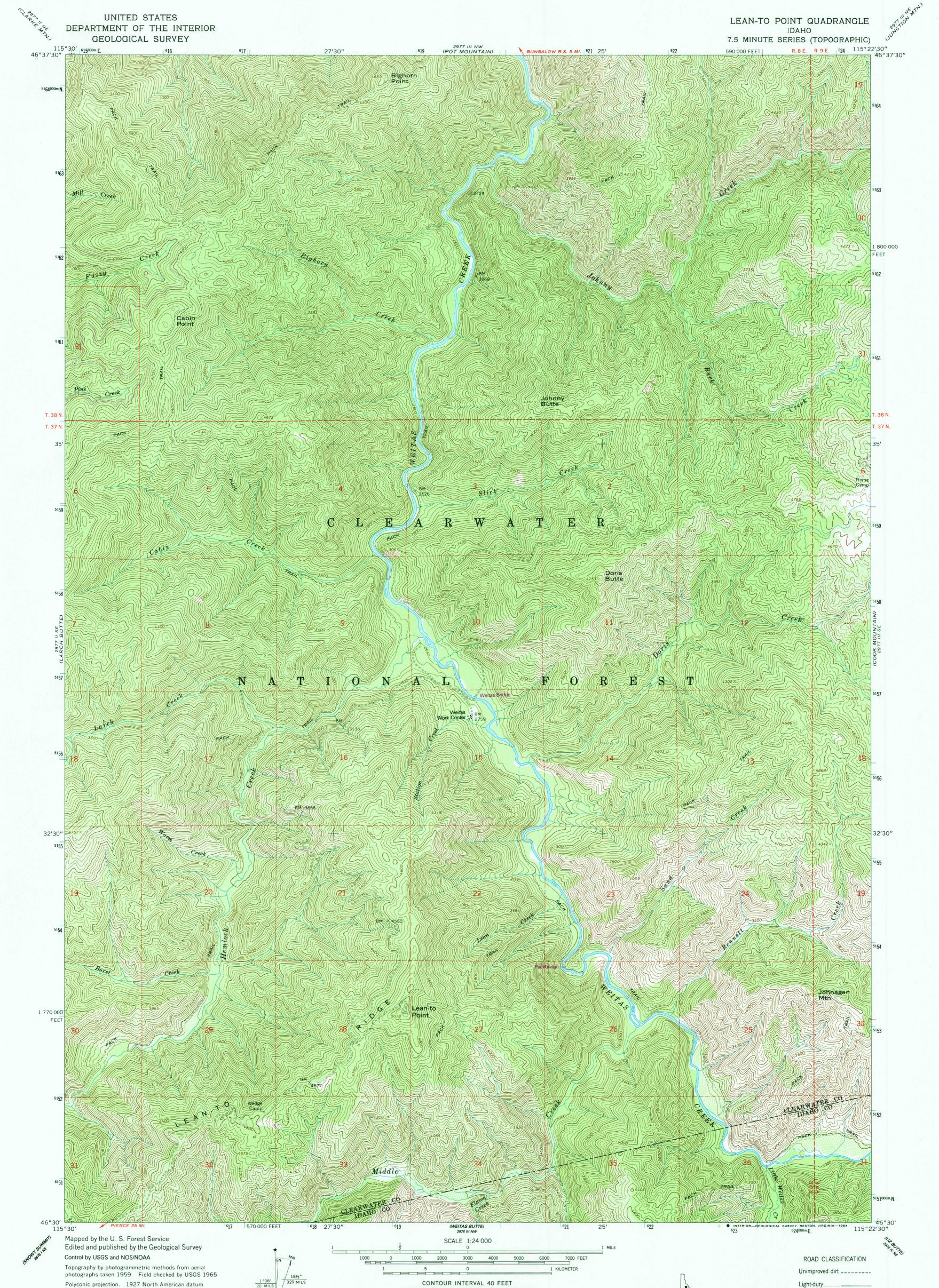
Polyconic projection. 1927 North American datum 10,000-foot grid based on Idaho coordinate system, west zone 1000-meter Universal Transverse Mercator grid ticks, zone 11, shown in blue To place on the predicted North American Datum 1983 move the projection lines 14 meters north and 74 meters east as shown by dshed corner ticks Where omitted, land lines have not been established There may be private inholdings within the boundaries of the National or State reservations shown on this map
