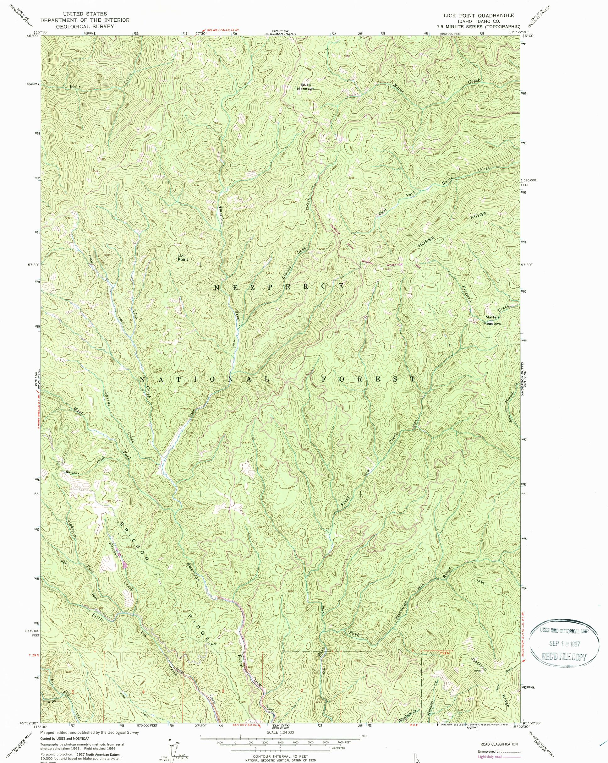
Polyconic projection. 1927 North American Datum 10,000-foot grid based on Idaho coordinate system, west zone 1000-meter Universal Transverse Mercator grid ticks, zone 11, shown in blue Where omitted, land lines have not been established To place on the predicted North American Datum 1983 move the projection lines 15 meters north and 74 meters east as shown by dashed corner ticks There may be private inholdings within the boundaries of the National or State reservations shown on this map
