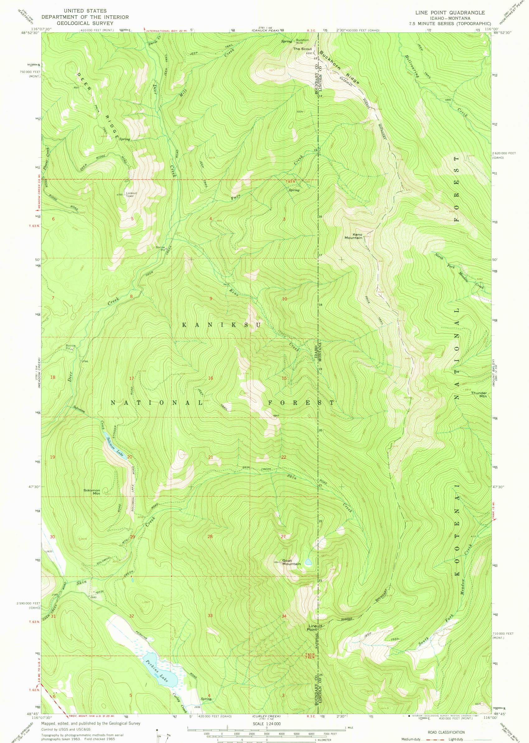
Polyconic projection. 1927 North American datum 10,000-foot grids based on Idaho coordinate system, 0°42' 12 MILS west zone, and Montana coordinate system, north zone 1000-meter Universal Transverse Mercator grid ticks, zone 11, shown in blue To place on the predicted North American Datum 1983, the resistion lines 12 meters porth and UTM GRID AND 1965 MAGNETIC NORTH DECLINATION AT CENTER OF SHEET move the projection lines 12 meters north and 76 meters east as shown by dashed corner ticks
