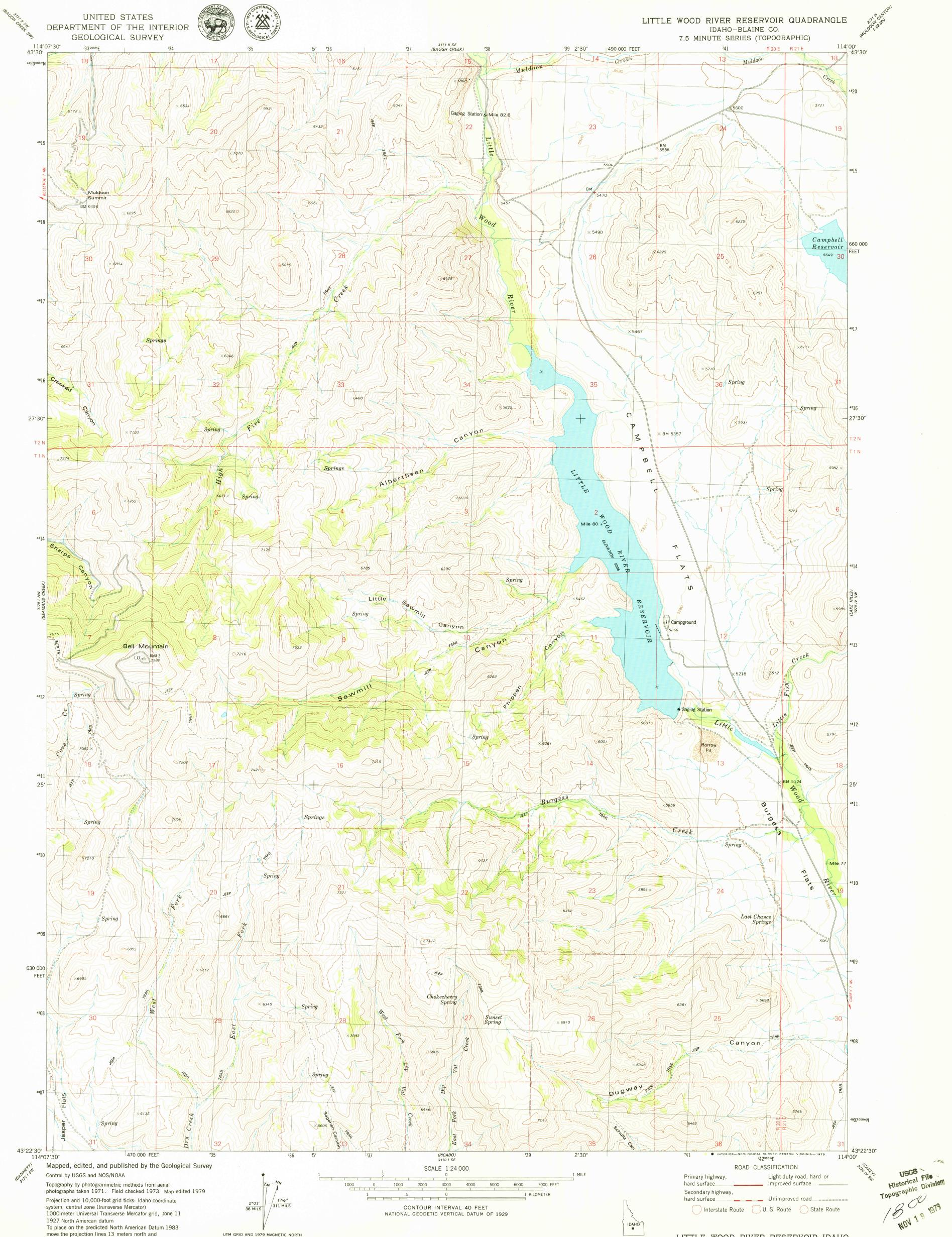
Projection and 10,000-foot grid ticks: Idaho coordinate system, central zone (transverse Mercator) 1000-meter Universal Transverse Mercator grid, zone 11 1927 North Amercan datum To place on the predicted North American Datum 1983 move the projection lines 13 meters north and 71 meters east as shown by dashed corner ticks
