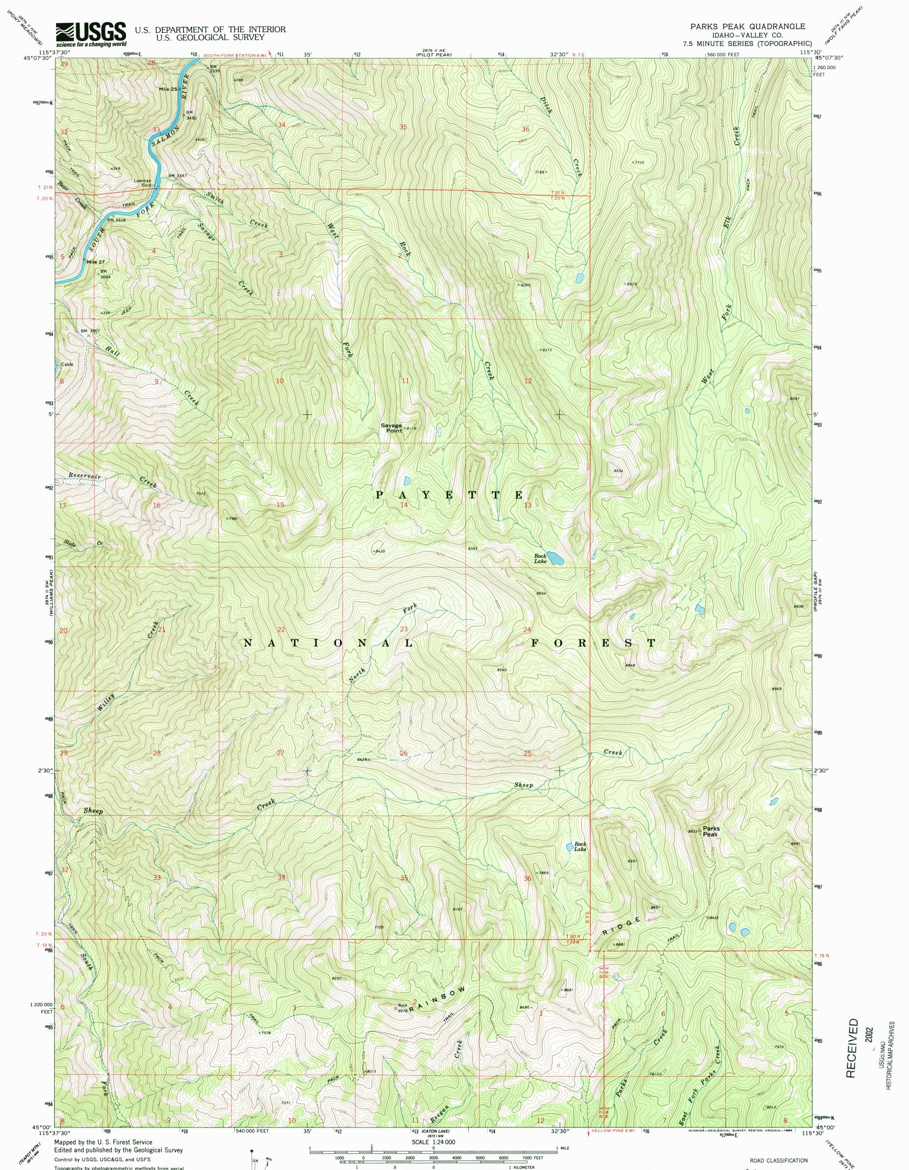
Topography by photogrammetric methods from aerial photographs taken 1964. Field checked by USGS 1969 Polyconic projection. 1927 North American datum 10,000-foot grid based on Idaho coordinate system, west zone 1000-meter Universal Transverse Mercator grid ticks, zone 11, shown in blue To place on the predicted North American Datum 1983 move the projection lines 15 meters north and
