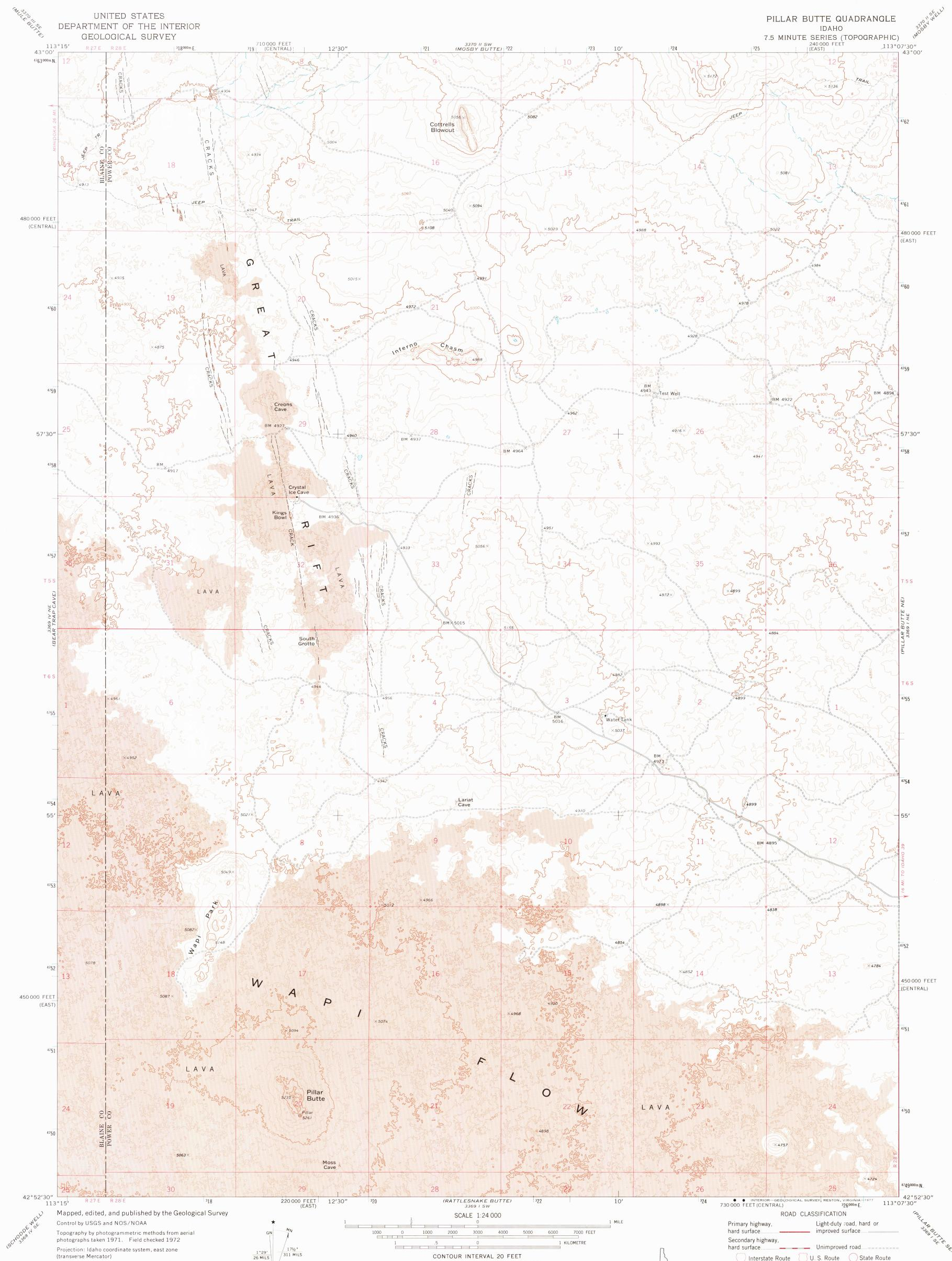
(transverse Mercator) 10,000-foot grid ticks based on Idaho coordinate system, east and central zones 1000-metre Universal Transverse Mercator grid ticks, UTM GRID AND 1972 MAGNETIC NORTH DECLINATION AT CENTER OF SHEET zone 12, shown in blue. 1927 North American datum Fine red dashed lines indicate selected fence lines
