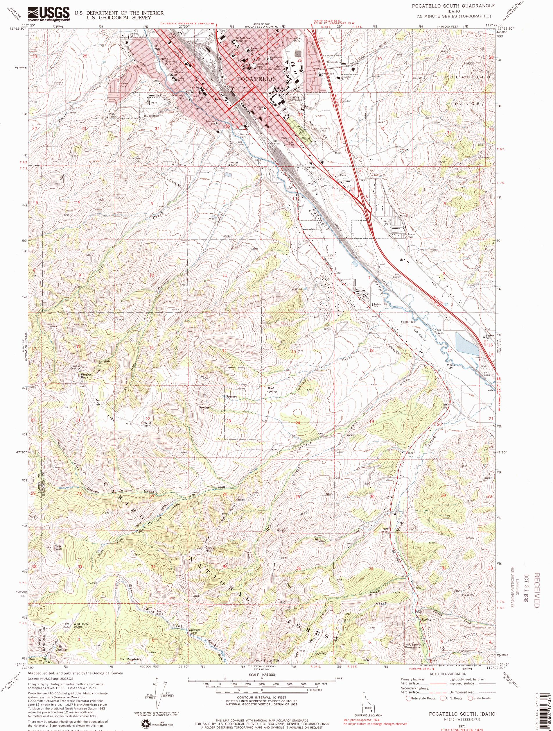
1000-meter Universal Transverse Mercator grid ticks, zone 12, shown in blue. 1927 North American datum To place on the predicted North American Datum 1983 move the projection lines 12 meters north and 67 meters east as shown by dashed corner ticks
