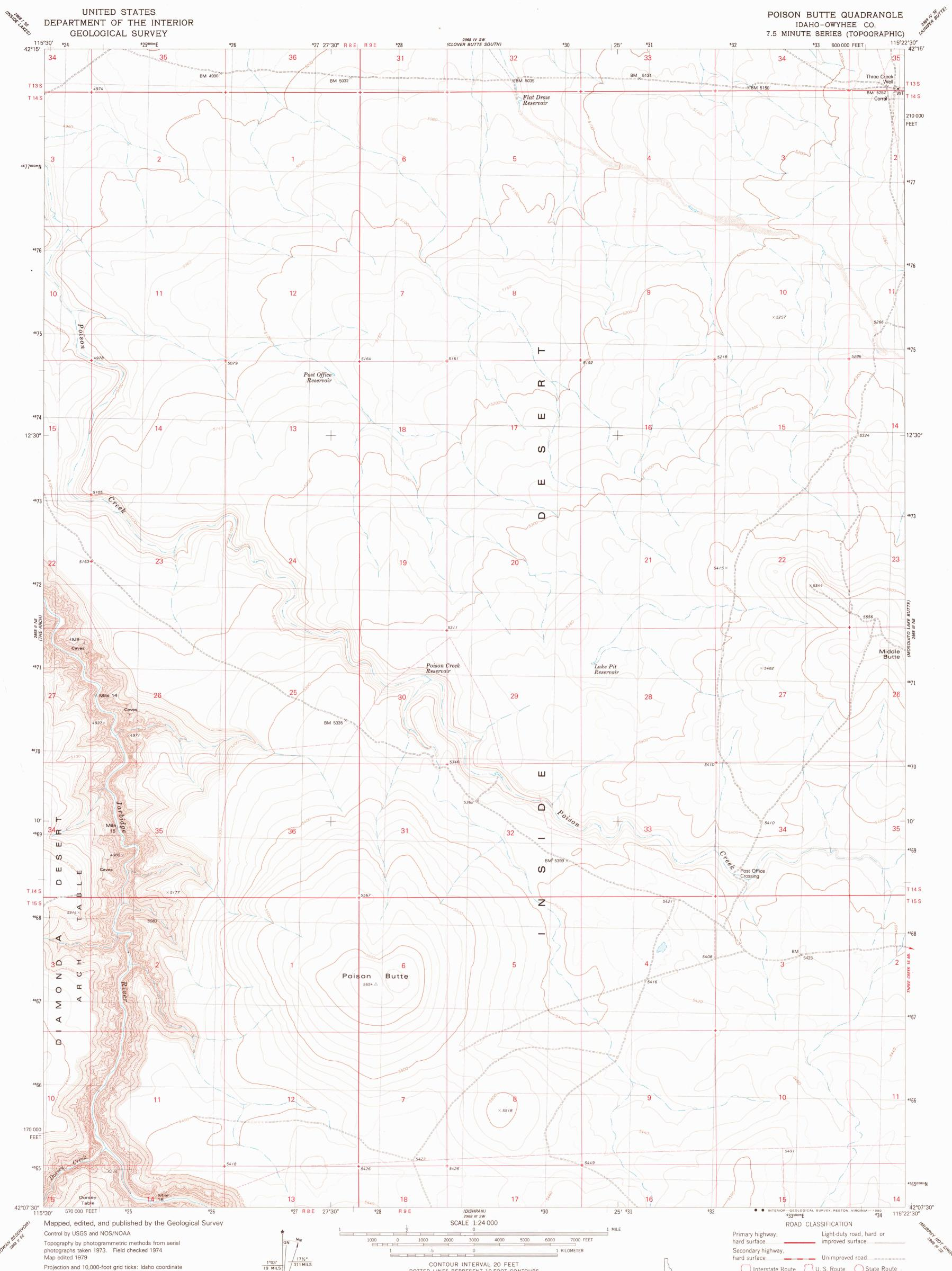
Projection and 10,000-foot grid ticks: Idaho coordinate system, west zone (transverse Mercator) 1000-meter Universal Transverse Mercator grid, zone 11 1927 North American datum To place on the predicted North American Datum 1983 move the projection lines 14 meters north and 75 meters east as shown by dashed corner ticks Fine red dashed lines indicate selected fence and field lines where generally visible on aerial photographs This information is unchecked
