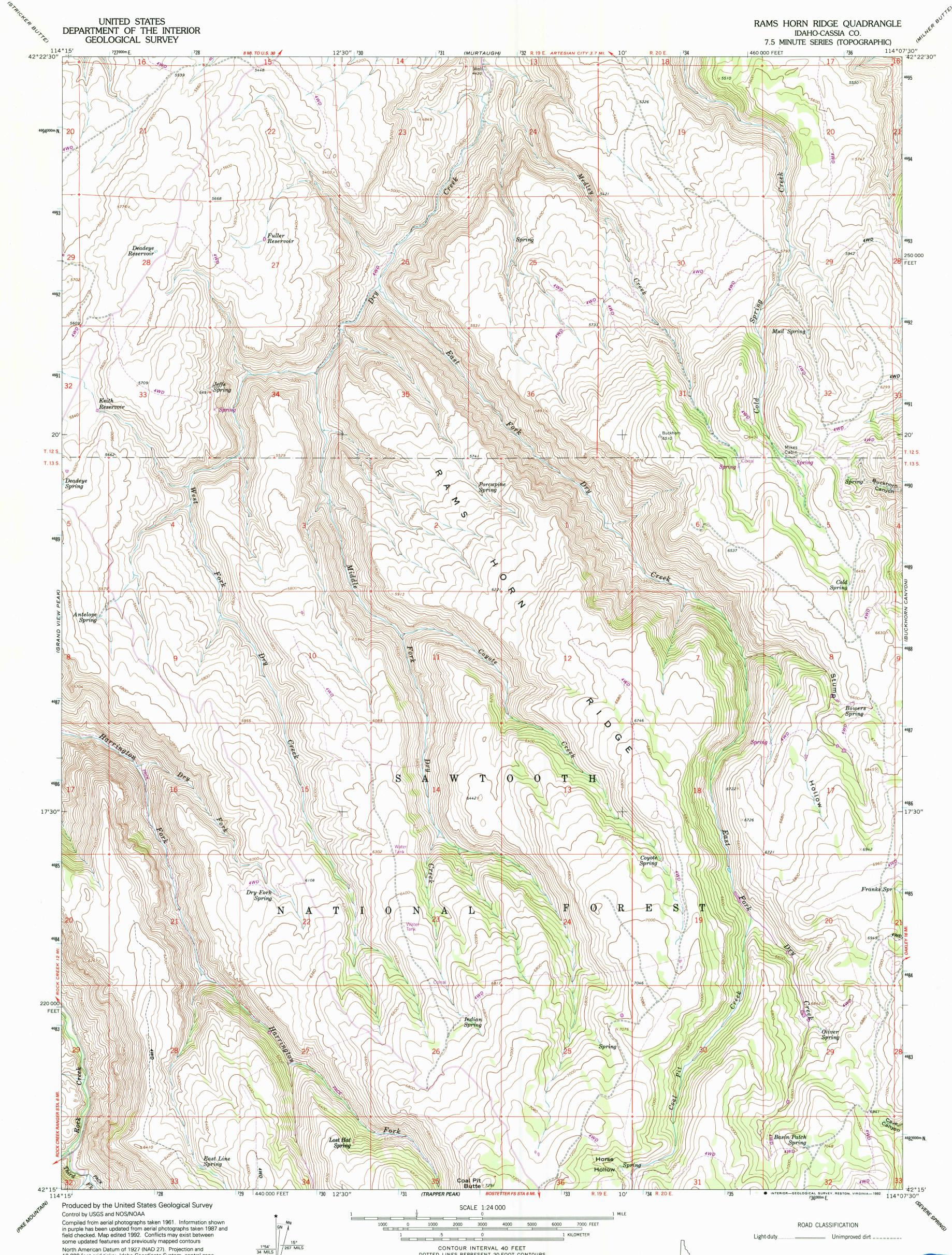
North American Datum of 1927 (NAD 27). Projection and 10,000-foot grid ticks: Idaho Coordinate System, central zone (Transverse Mercator). 1000-meter Universal Transverse Mercator grid ticks, zone 11, shown in blue The difference between NAD 27 and North American Datum of 1983 (NAD 83) for 7.5 minute intersections is given in USGS Bulletin 1875. The NAD 83 is shown by dashed corner ticks
