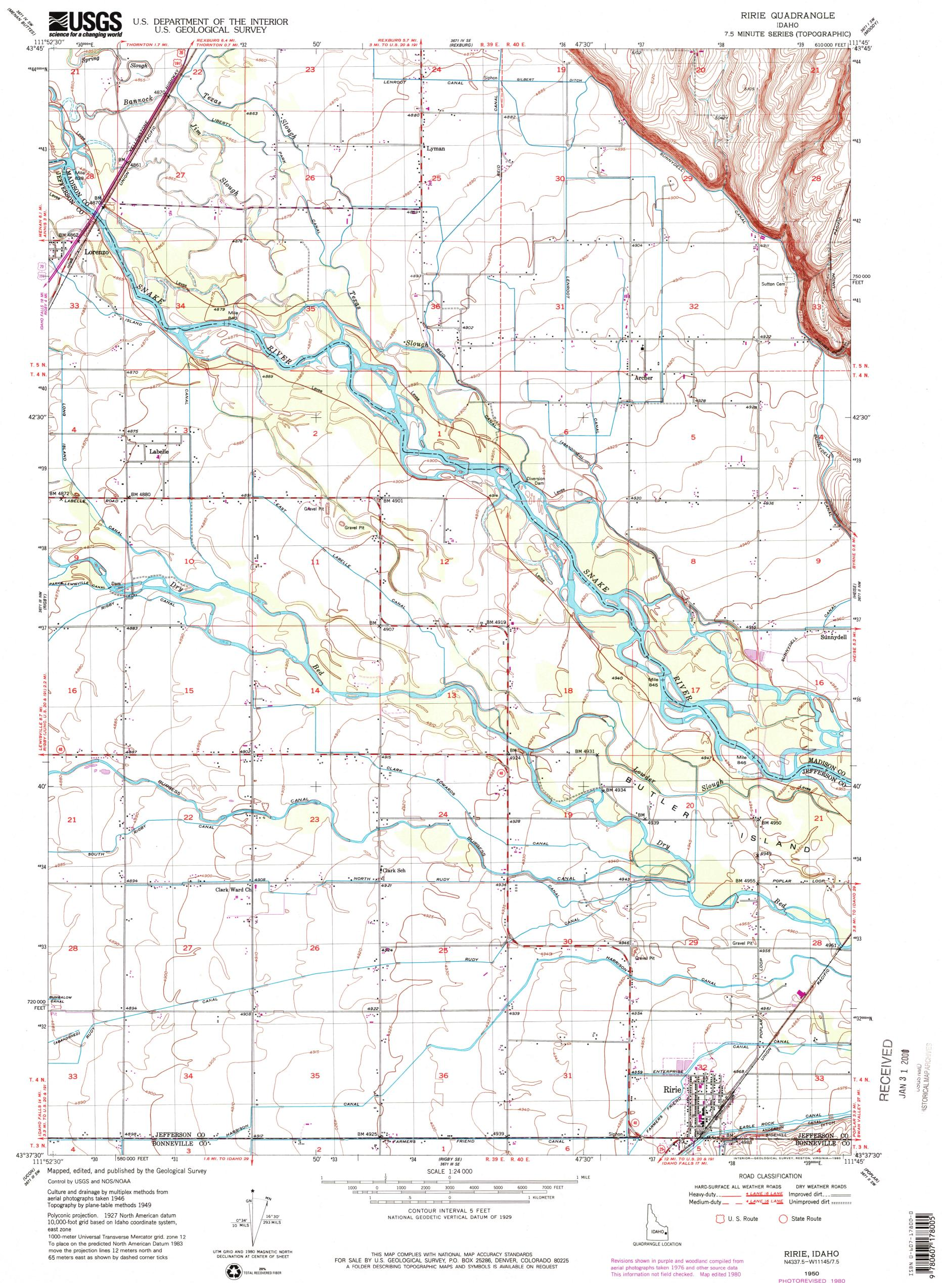
Polyconic projection. 1927 North American datum 10,000-foot grid based on Idaho coordinate system, east zone 1000-meter Universal Transverse Mercator grid. zone 12 To place on the predicted North American Datum 1983 move the projection lines 12 meters north and 65 meters east as shown by dashed corner ticks
