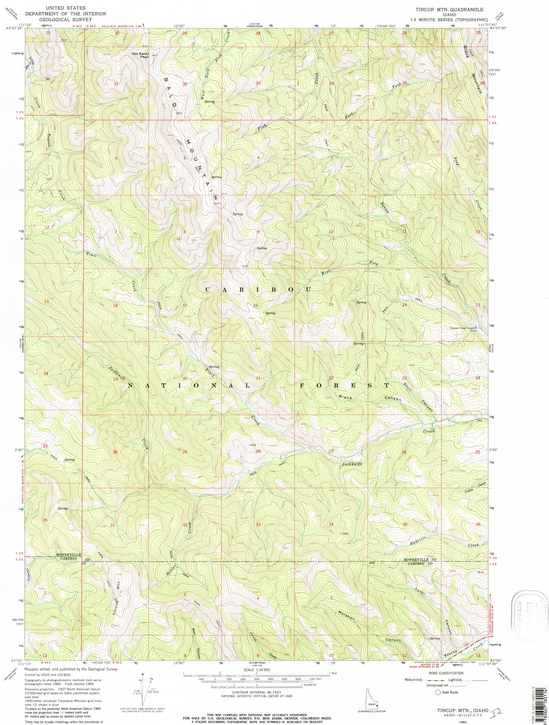
10,000-foot grid based on Idaho coordinate system, east zone 1000-meter Universal Transverse Mercator grid ticks, zone 12, shown in blue To place on the predicted North American Datum 1983 UTM GRID AND 1966 MAGNETIC NORTH DECLINATION AT CENTER OF SHEET move the projection lines 11 meters north and 63 meters east as shown by dashed corner ticks There may be private inholdings within the boundaries of
