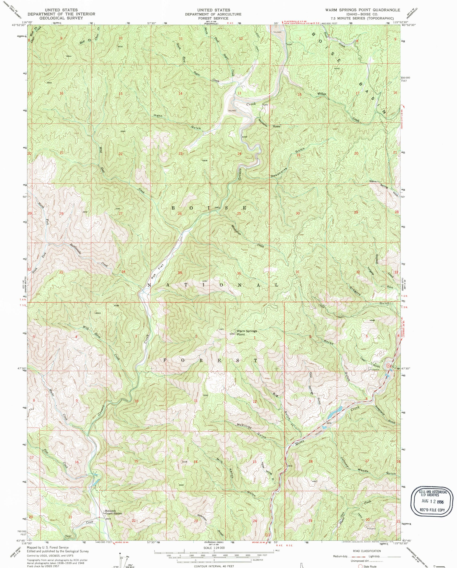
Field check by USGS 1957 Polyconic projection. 1927 North American datum 10,000-foot grid based on Idaho coordinate system, west zone 1000-meter Universal Transverse Mercator grid ticks, zone 11, shown in blue To place on the predicted North American Datum 1983, move the projection lines 15 meters north and 76 meters east as shown by dashed corner ticks
