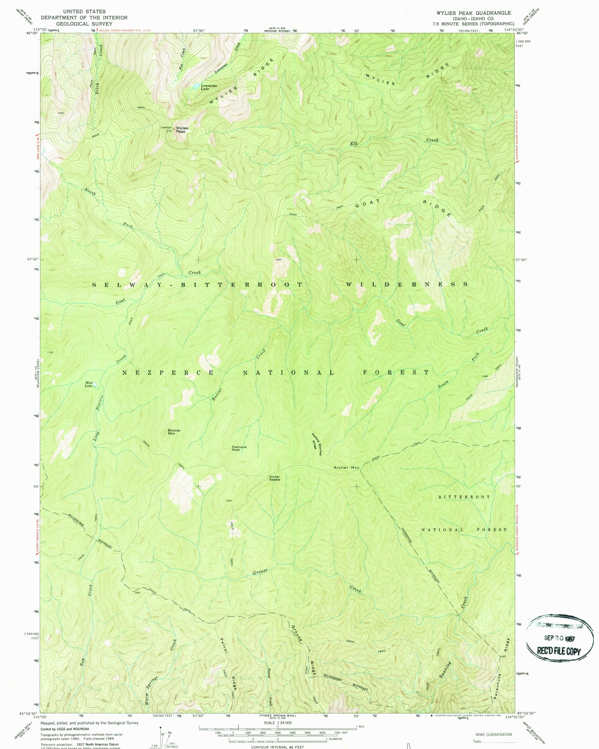
10,000-foot grid based on Idaho coordinate system, west zone 1000-meter Universal Transverse Mercator grid ticks, zone 11, shown in blue To place on the predicted North American Datum 1983, move the projection lines 14 meters north and 73 meters east as shown by dashed corner ticks Land lines have not been established in this area There may be private inholdings within the boundaries of the National or State reservations shown on this map
