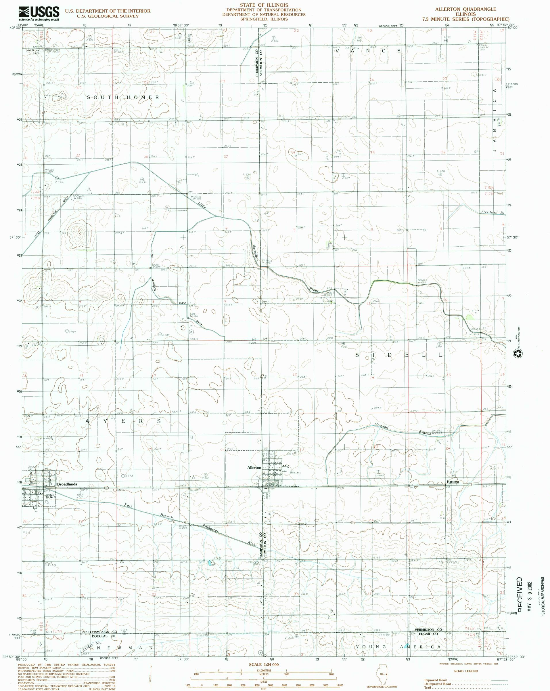
UTM GRID DECLINATION .... .....0°36' WEST North American Datum of 1983 (NAD 83) is shown by dashed corner ticks. The values of the shift between NAD 27 and NAD 83 for 7.5-minute intersections are obtainable from National Geodetic Survey NADCON software
