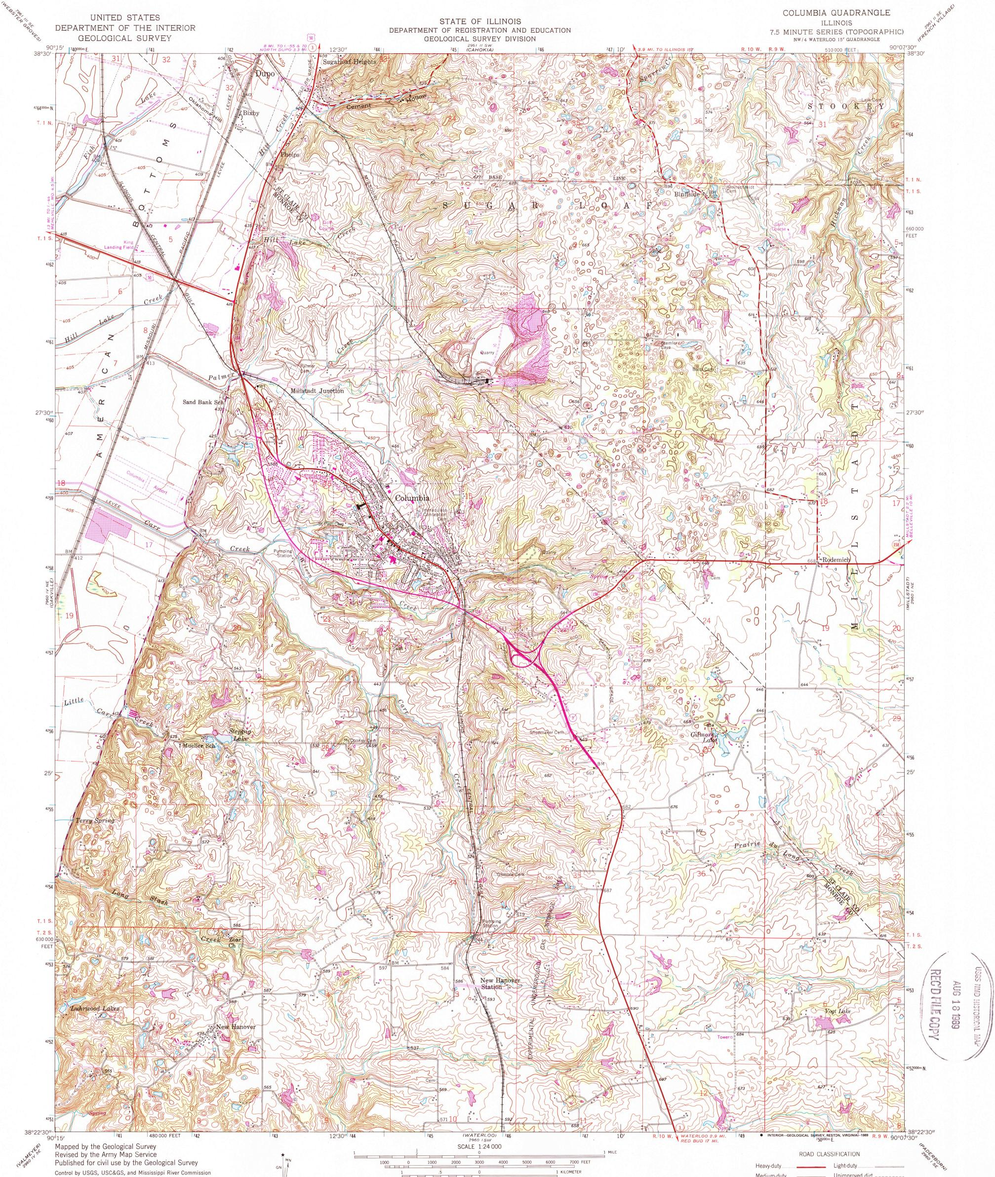
Culture and drainage in part compiled from aerial photographs taken 1946. Topography from planetable surveys by the Geological Survey 1949. Planimetric detail revised from aerial photographs taken 1952. Field check 1955
