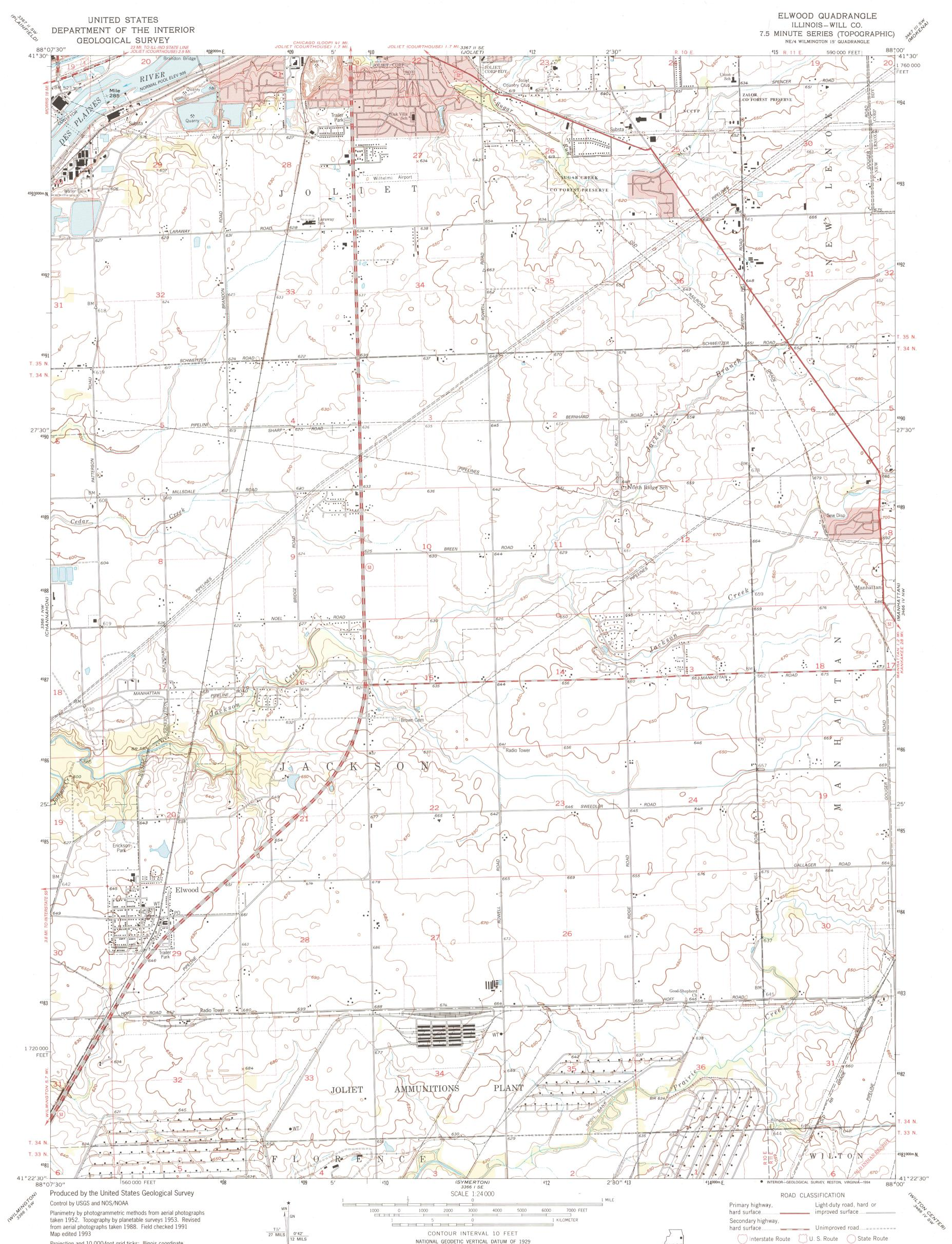
Projection and 10,000-foot grid ticks: Illinois coordinate system, east zone (transverse Mercator) 1000-meter Universal Transverse Mercator grid ticks, zone 16, shown in blue 1927 North American Datum (NAD 27)
