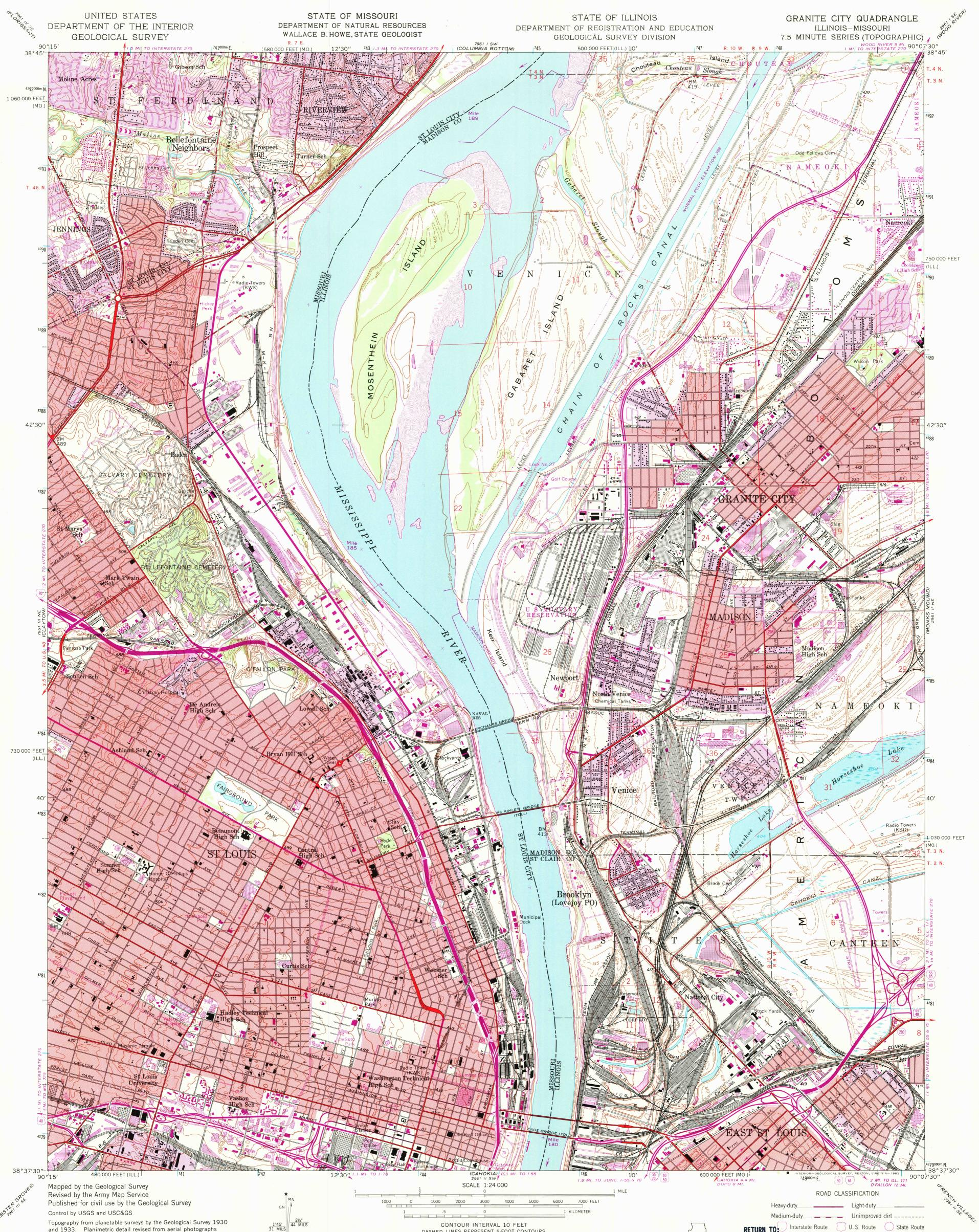
Topography from planetable surveys by the Geological Survey 1930 and 1933. Planimetric detail revised from aerial photographs taken 1952. Field check 1954
