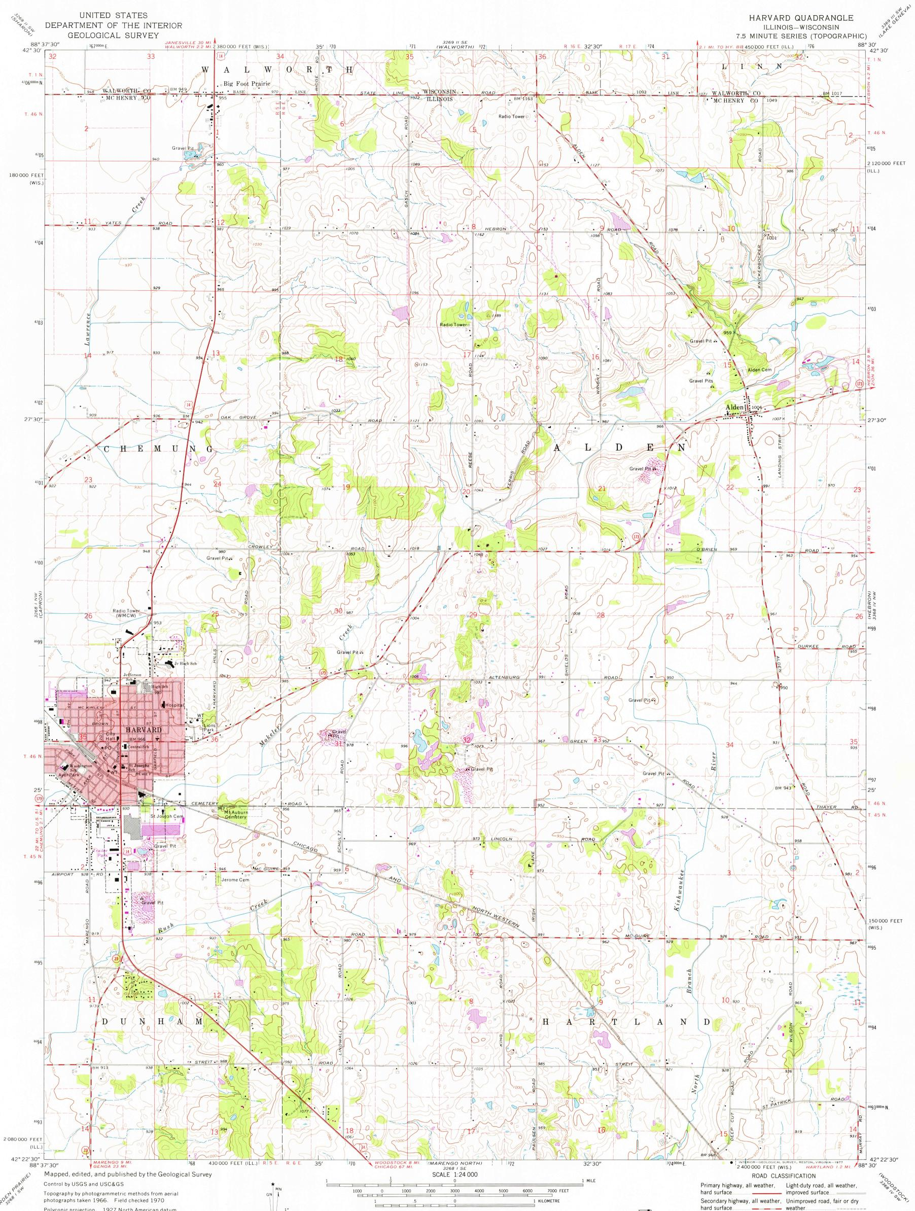
Polyconic projection. 1927 North American datum 10,000-foot grids based on Illinois coordinate system, east zone and Wisconsin coordinate system, south zone 1000-metre Universal Transverse Mercator grid ticks, zone 16, shown in blue Red tint indicates area in which only landmark buildings are shown
