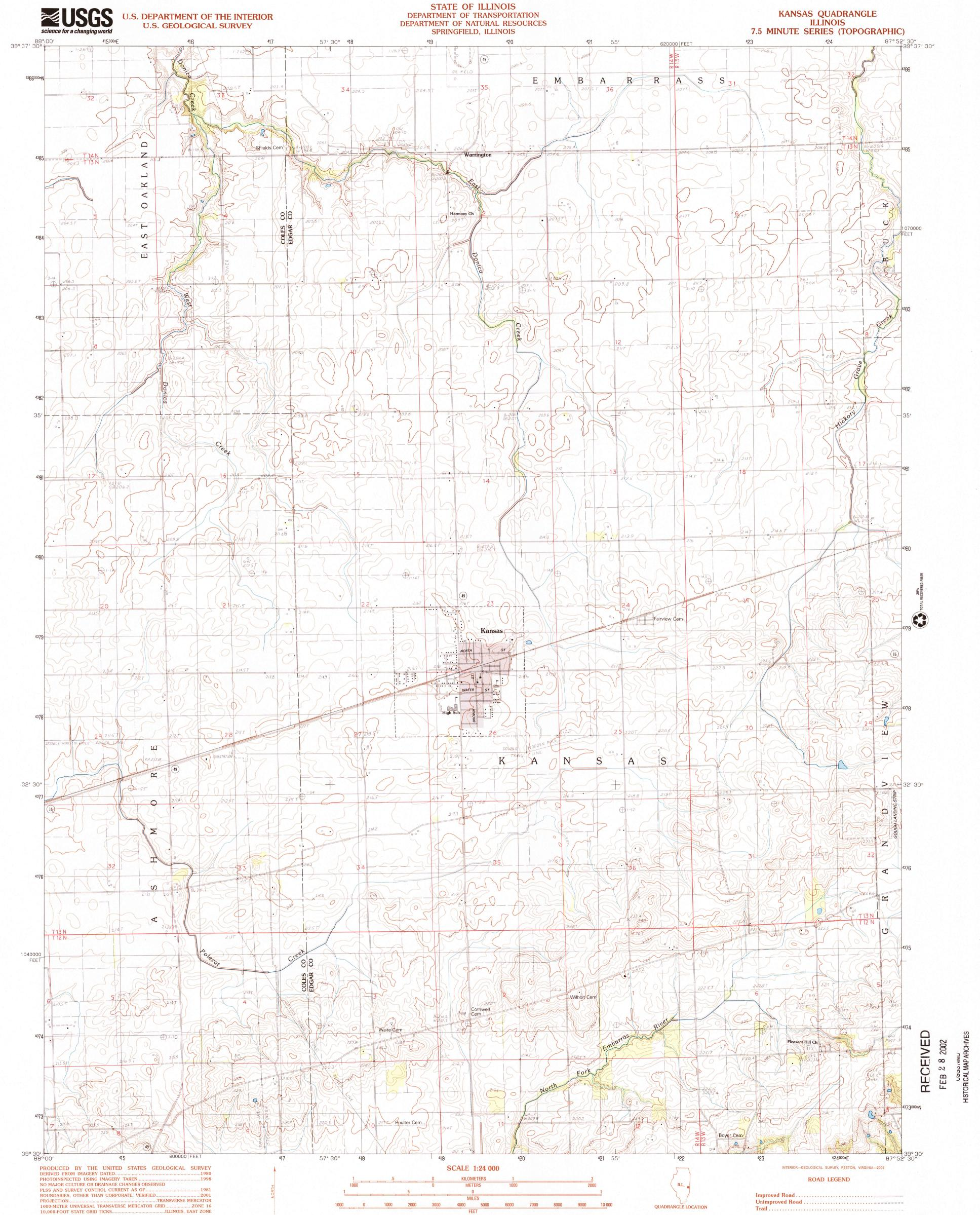
UTM GRID DECLINATION...... 2002 MAGNETIC NORTH DECLINATION...... .....0°36' WEST ...2°00' WEST VERTICAL DATUM......NATIONAL GEODETIC VERTICAL DATUM OF 1929 HORIZONTAL DATUM.....NORTH AMERICAN DATUM OF 1927 (NAD 27) North American Datum of 1983 (NAD 83) is shown by dashed corner ticks. The values of the shift between NAD 27 and NAD 83 for 7.5-minute intersections are obtainable from National Geodetic Survey NADCON software
