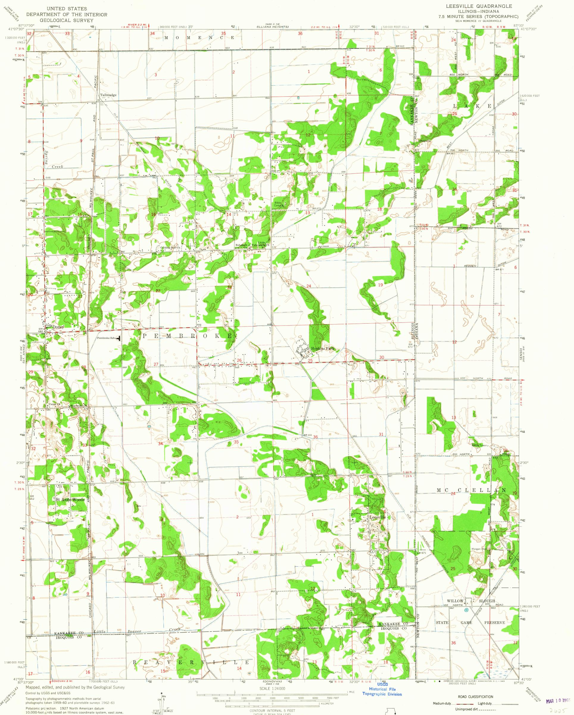
Polyconic projection. 1927 North American datum 10,000-foot grids based on Illinois coordinate system, east zone, and Indiana coordinate system, west zone 1000-meter Universal Transverse Mercator grid ticks, zone 16, shown in blue
