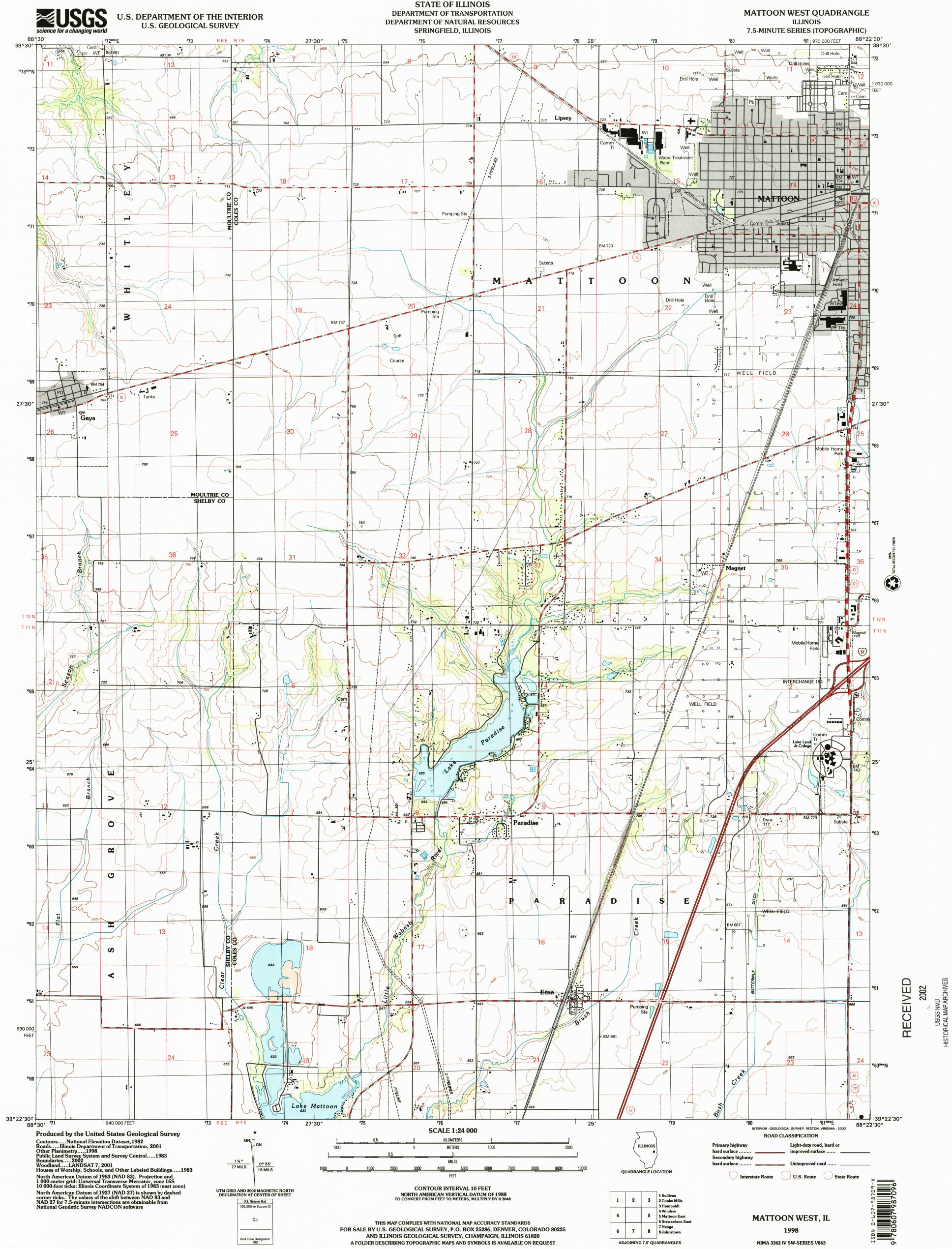
North American Datum of 1983 (NAD 83). Projection and 1 000-meter grid: Universal Transverse Mercator, zone 16S 10 000-foot ticks: Illinois Coordinate System of 1983 (east zone) North American Datum of 1927 (NAD 27) is shown by dashed corner ticks. The values of the shift between NAD 83 and NAD 27 for 7.5-minute intersections are obtainable from National Geodetic Survey NADCON software
