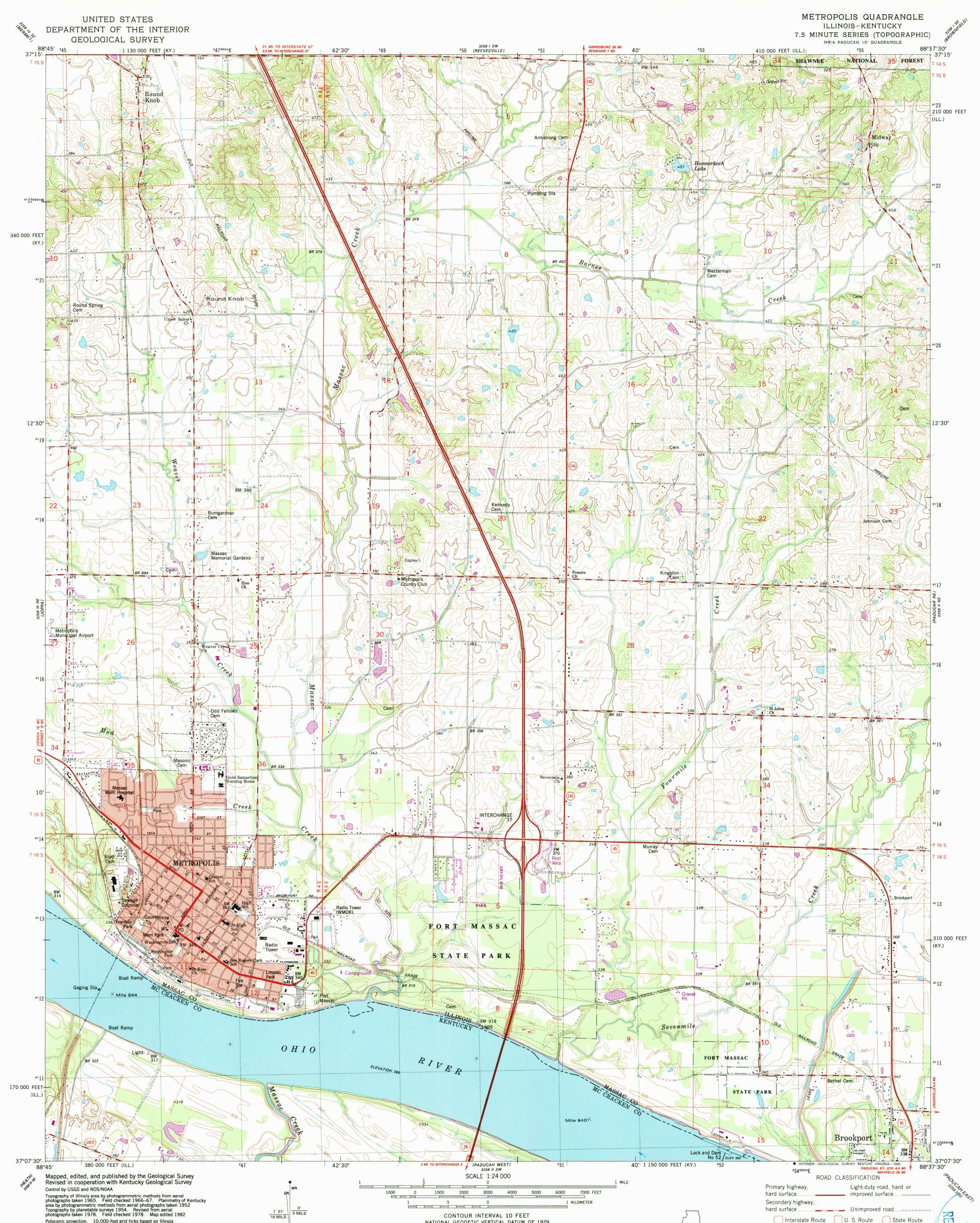
Polyconic projection. 10,000-foot grid ticks based on Illinois coordinate system, east zone, and Kentucky coordinate system, south zone 1000-meter Universal Transverse Mercator grid, zone 16 1927 North American Datum To place on the predicted North American Datum 1983 move the projection lines 4 meters south and 5 meters east as shown by dashed corner ticks Red tint indicates area in which only landmark buildings are shown
