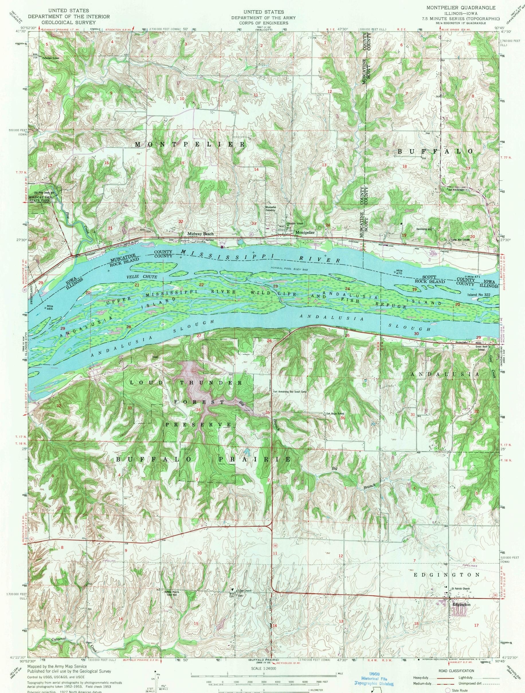
Polyconic projection. 1927 North American datum 10,000-foot grids based on Illinois coordinate system, west zone, and Iowa coordinate system, south zone 1000-meter Universal Transverse Mercator grid ticks, zone 15, shown in blue
