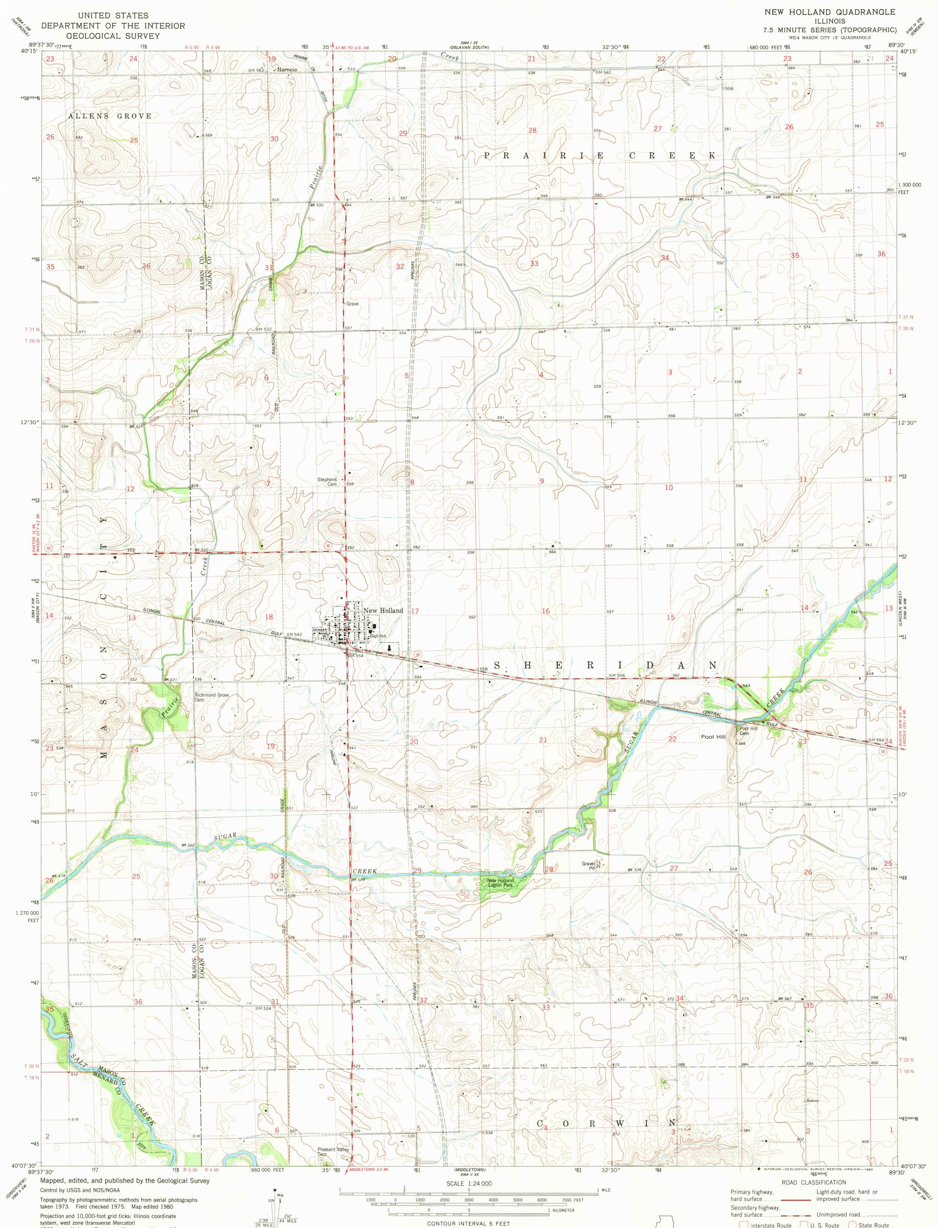
system, west zone (transverse Mercator) 1000-meter Universal Transverse Mercator grid, zone 16 1927 North American Datum To place on the predicted North American Datum 1983 move the projection lines 8 meters east as shown by dashed corner ticks
