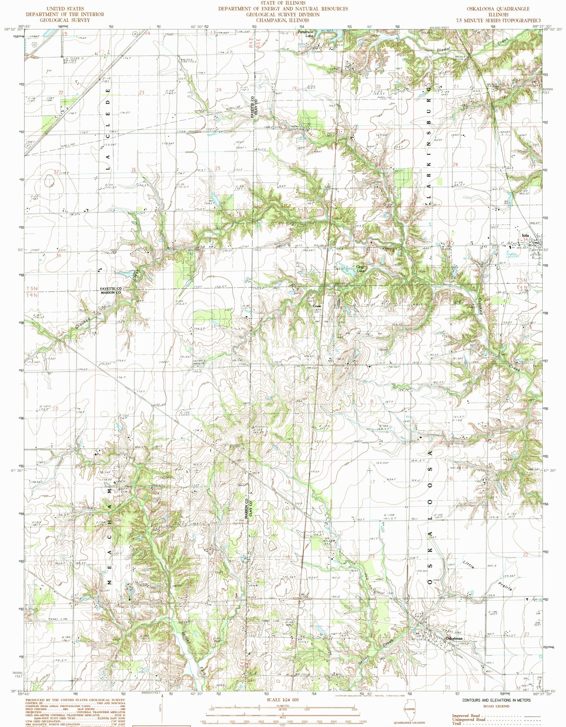
VERTICAL DATUM ...... NATIONAL GEODETIC VERTICAL DATUM OF 1929 HORIZONTAL DATUM ...... 1927 NORTH AMERICAN DATUM To place on the predicted North American Datum of 1983, move the projection lines as shown by dashed corner ticks (2 meters south and 5 meters east) There may be private inholdings within the boundaries of any Federal and State Reservations shown on this map No distinction made between houses, barns, and other buildings
