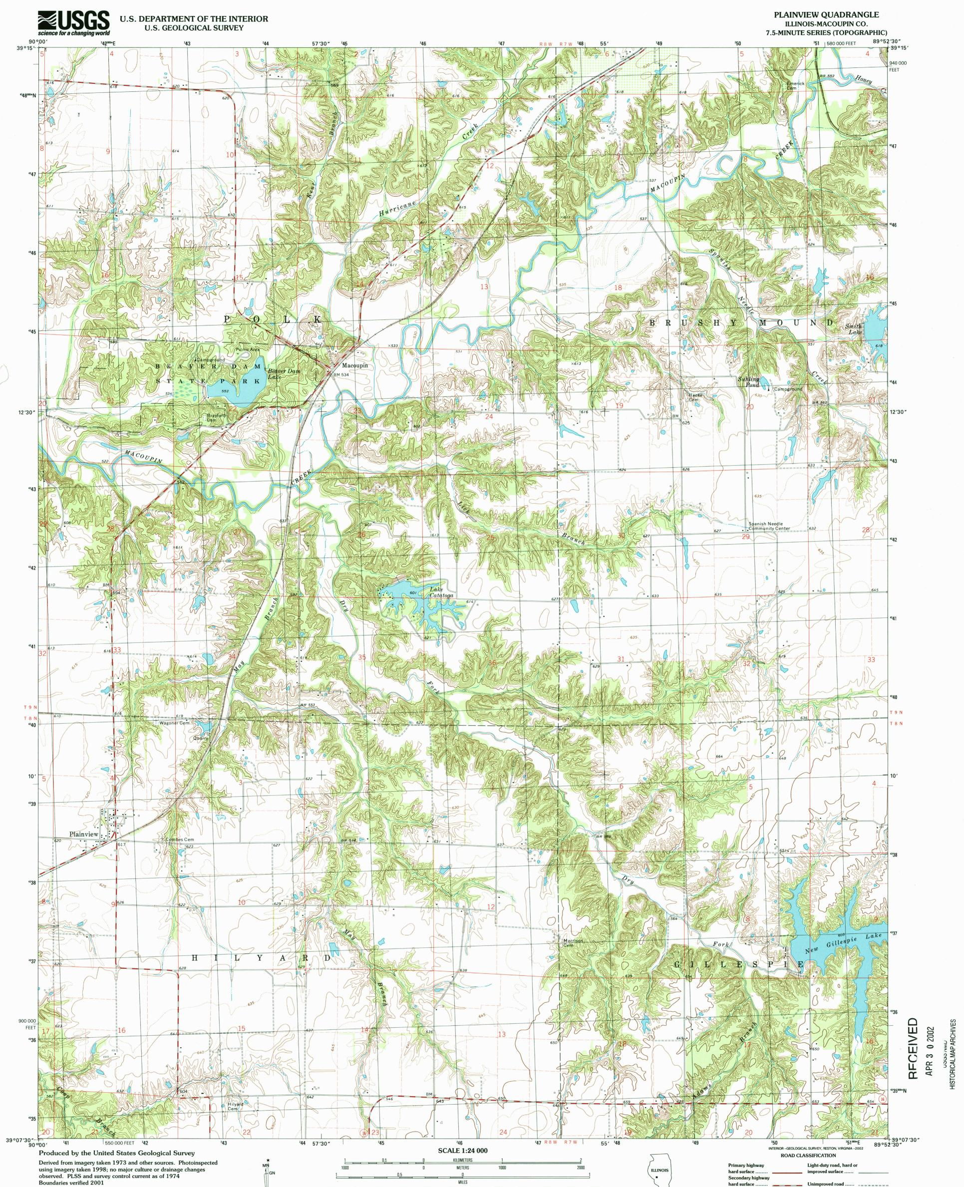
North American Datum of 1927 (NAD 27). Projection and 10 000-foot ticks: Illinois coordinate system, west zone (transverse Mercator) 1000-meter Universal Transverse Mercator grid, zone 16 North American Datum of 1983 (NAD 83) is shown by dashed corner ticks. The values of the shift between NAD 27 and NAD 83 for 7.5-minute intersections are obtainable from National Geodetic Survey NADCON software
