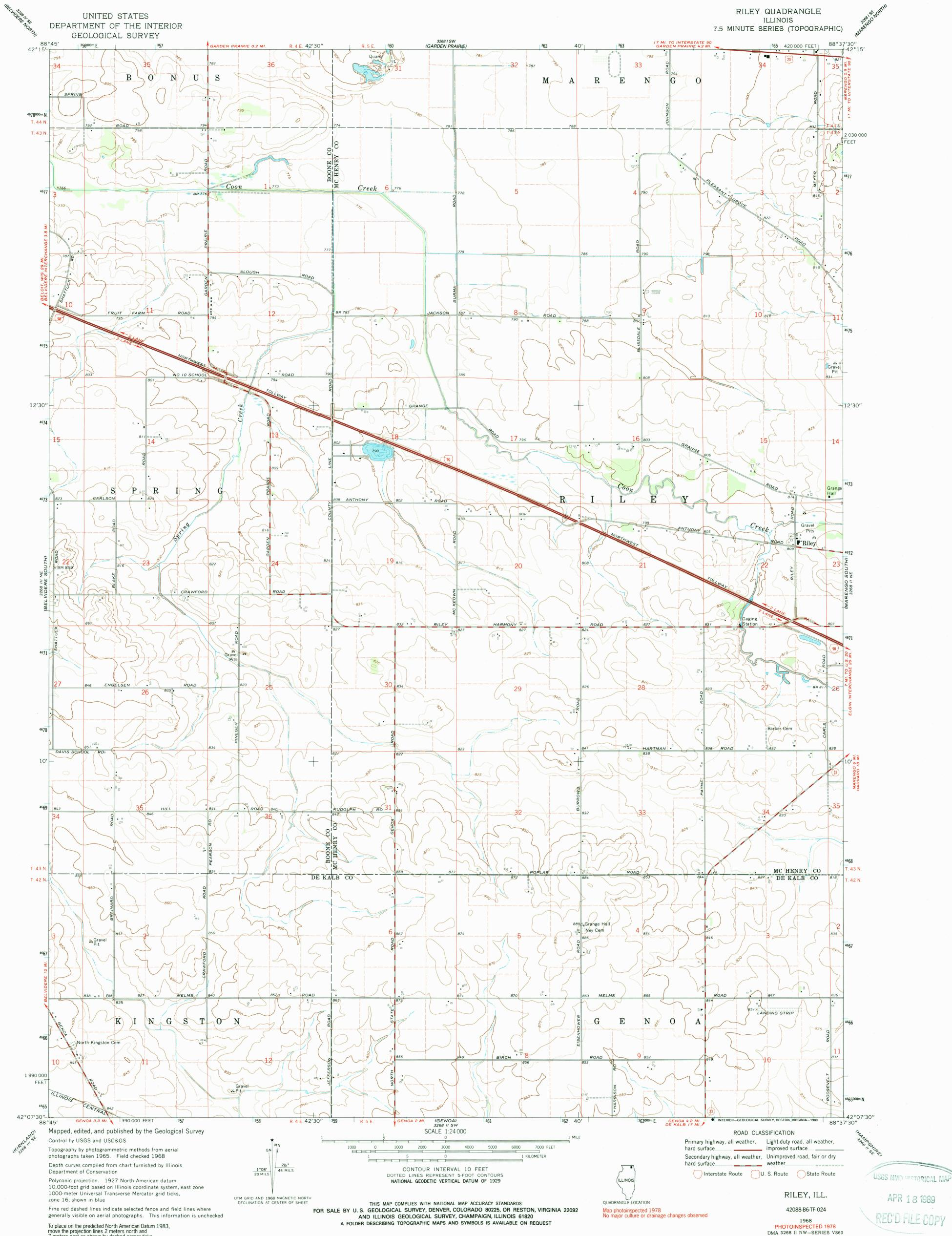
To place on the predicted North American Datum 1983, move the projection lines 2 meters north and 7 meters east as shown by dashed corner ticks
