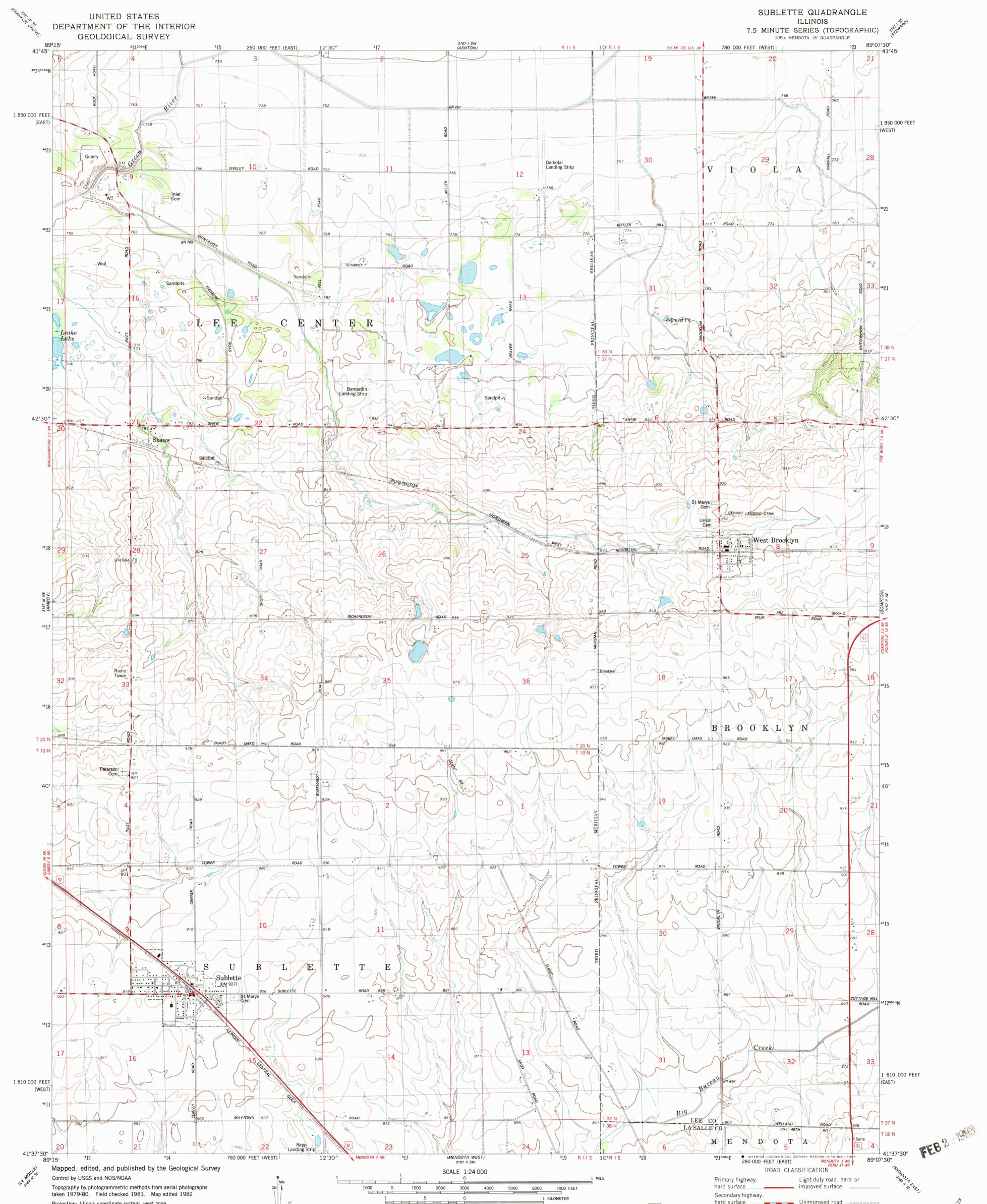
Projection: Illinois coordinate system, west zone (transverse Mercator) 10,000-foot grid ticks based on Illinois coordinate system, west and east zones 1000-meter Universal Transverse Mercator grid, zone 16 1927 North American Datum To place on the predicted North American Datum 1983 move the projection lines 2 meters north and 8 meters east as shown by dashed corner ticks Fine red dashed lines indicate selected fence and field lines where
