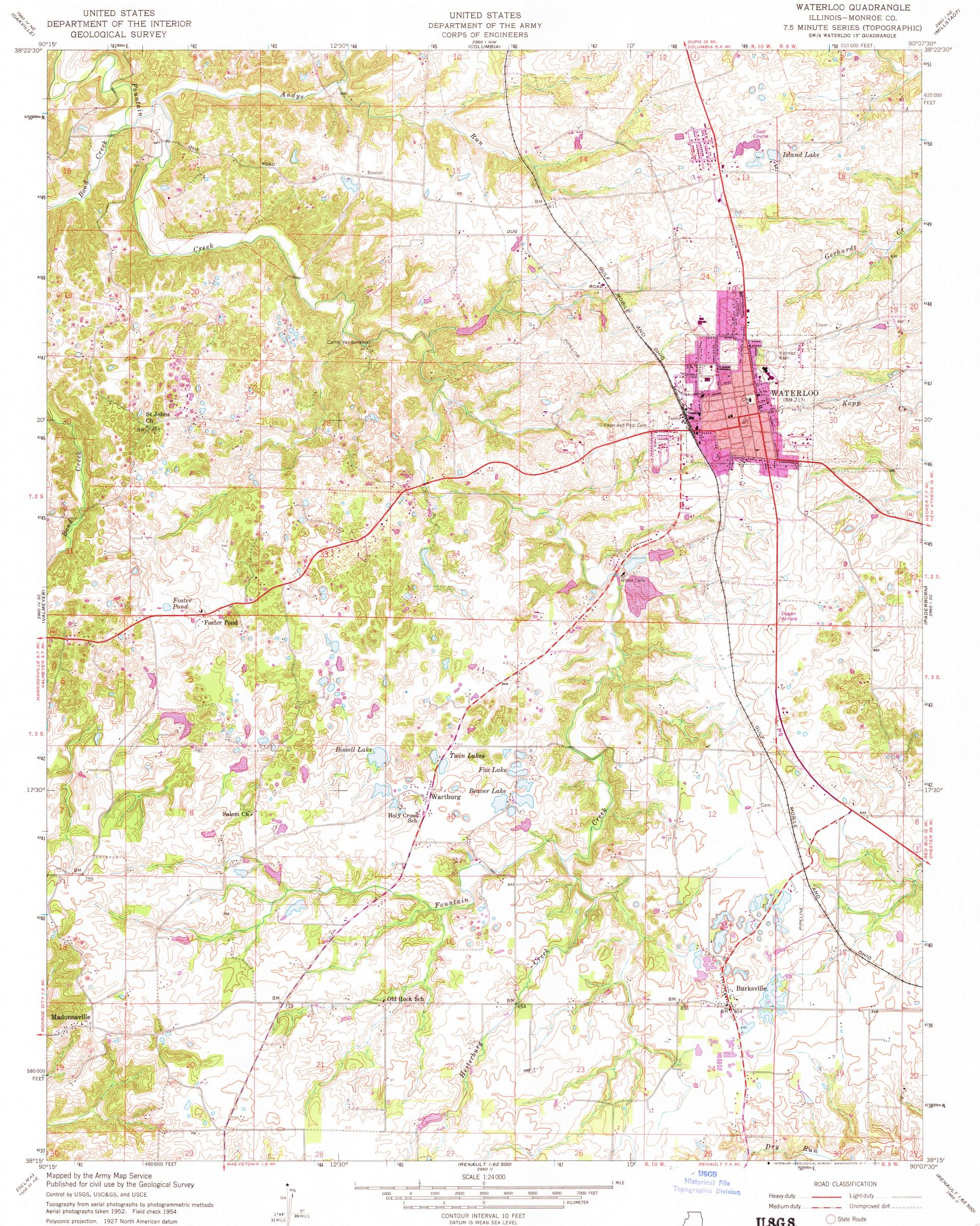
Polyconic projection. 1927 North American datum 10,000-foot grid based on Illinois coordinate system, west zone 1000-meter Universal Transverse Mercator grid ticks, zone 15, shown in blue
