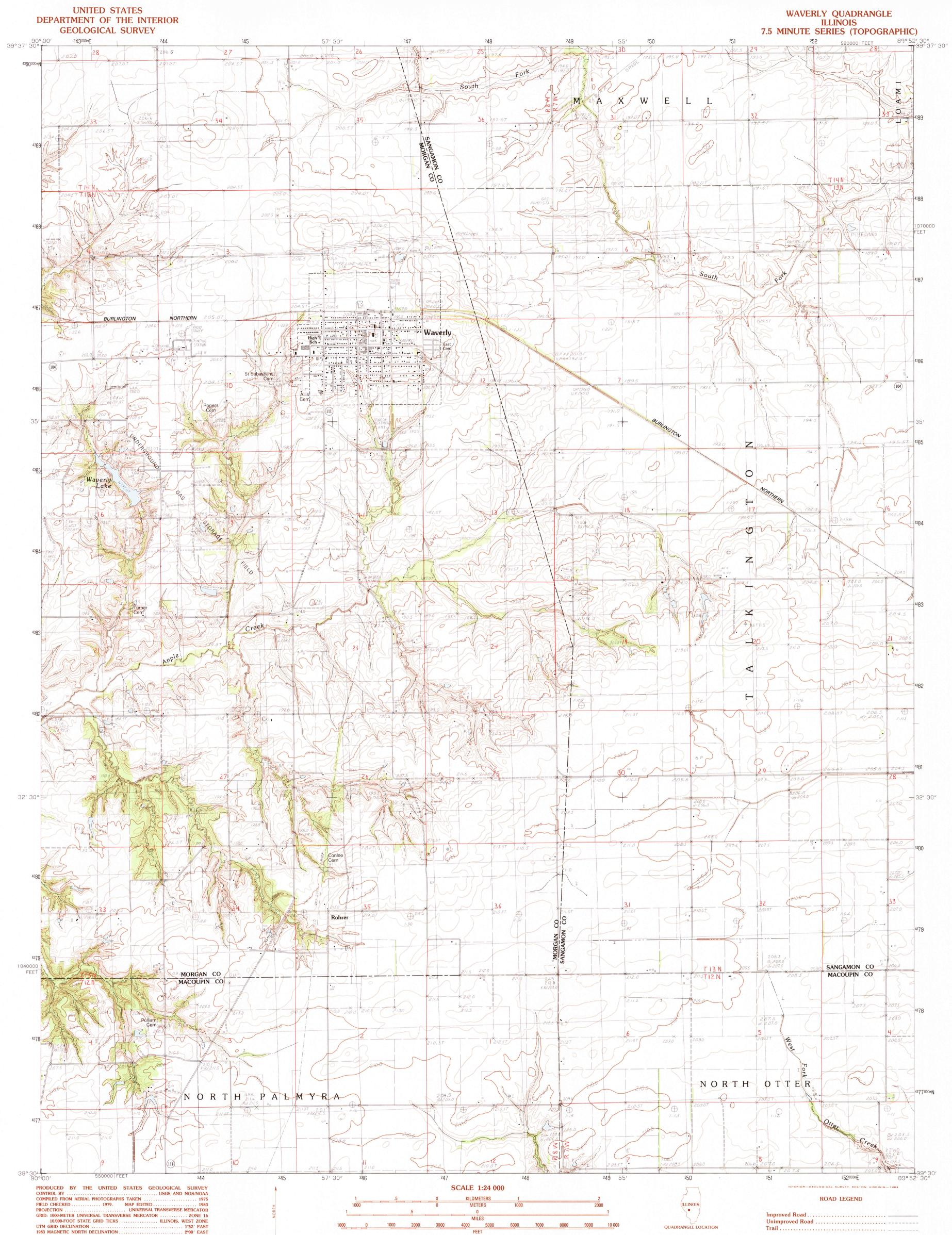
UTM GRID DECLINATION ..... 1°52' EAST To place on the predicted North American Datum of 1983, move the projection lines as shown by dashed corner ticks (1 meter south and 8 meters east) There may be private inholdings within the boundaries of any
