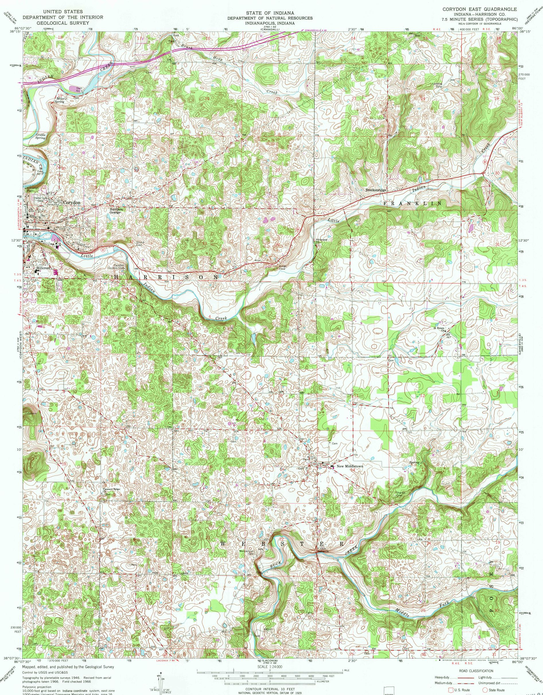
Polyconic projection 10,000-foot grid based on Indiana coordinate system, east zone 1000-meter Universal Transverse Mercator grid ticks, zone 16, shown in blue. 1927 North American Datum To place on the predicted North American Datum 1983 move the projection lines 3 meters south and 2 meters west as shown by dashed corner ticks
