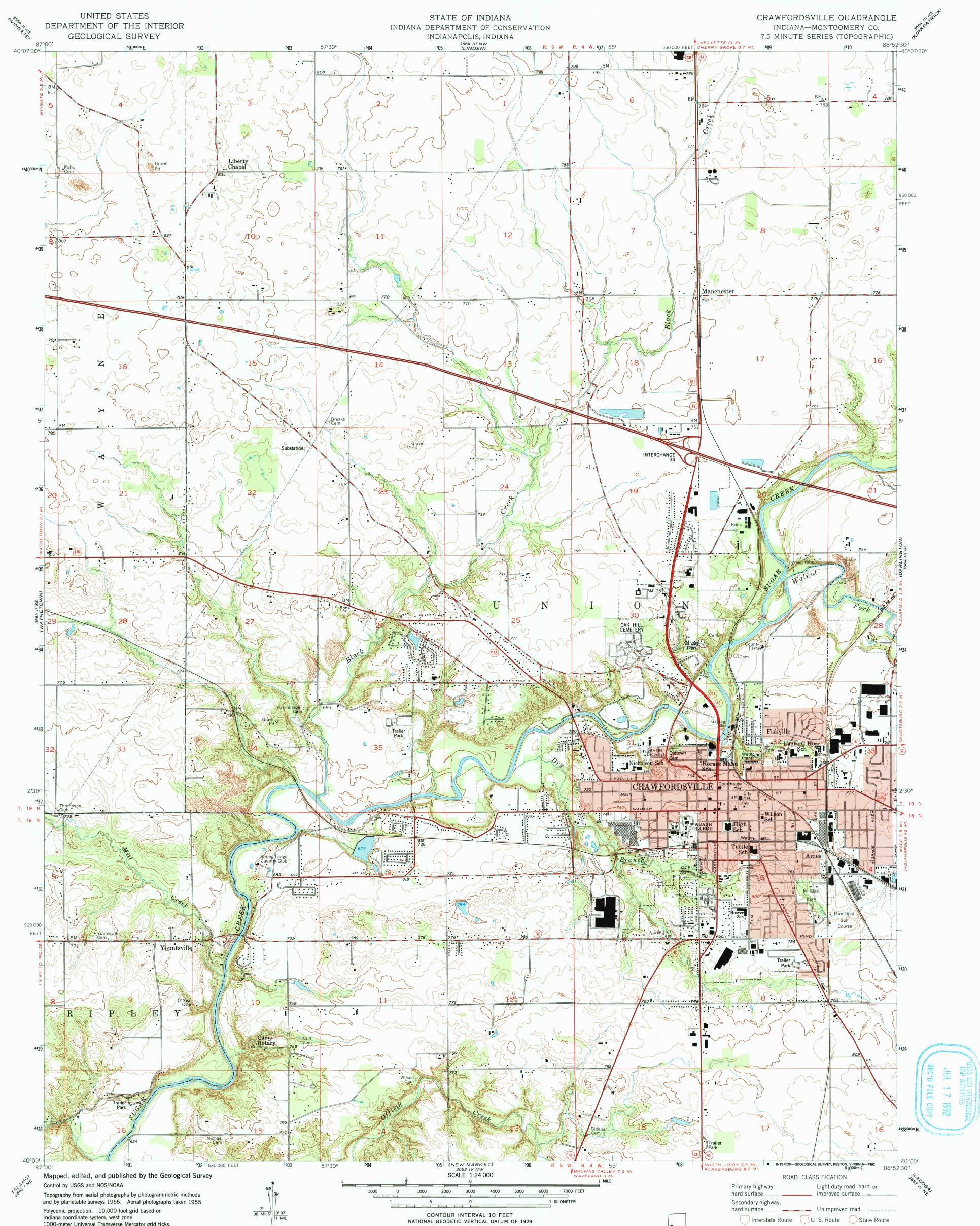
Indiana coordinate system, west zone 1000-meter Universal Transverse Mercator grid ticks, zone 16, shown in blue. 1927 North American Datum To place on the predicted North American Datum 1983 move the projection lines 1 meter south and 1 meter east as shown by dashed corner ticks UTM GRID AND 1992 MAGNETIC NORTH DECLINATION AT CENTER OF SHEET
