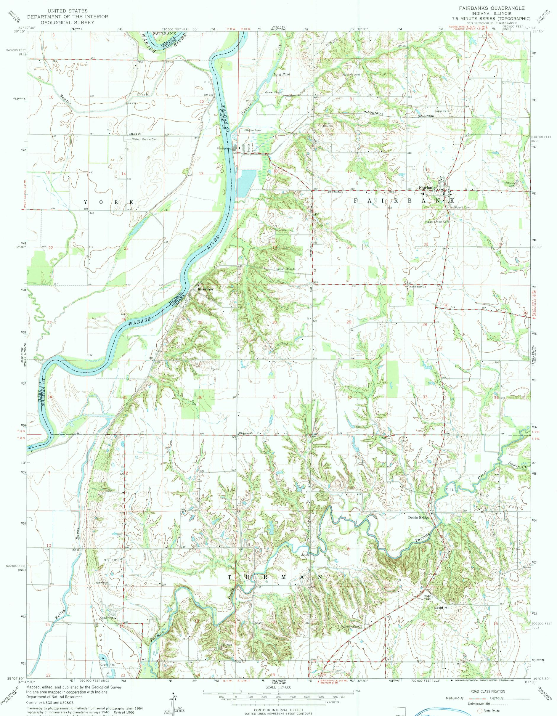
Planimetry by photogrammetric methods from aerial photographs taken 1964 Topography of Indiana area by planetable surveys 1940. Revised 1966 Topography of Illinois area by photogrammetric methods from aerial photographs taken 1956. Field checked 1957. Revised 1966
