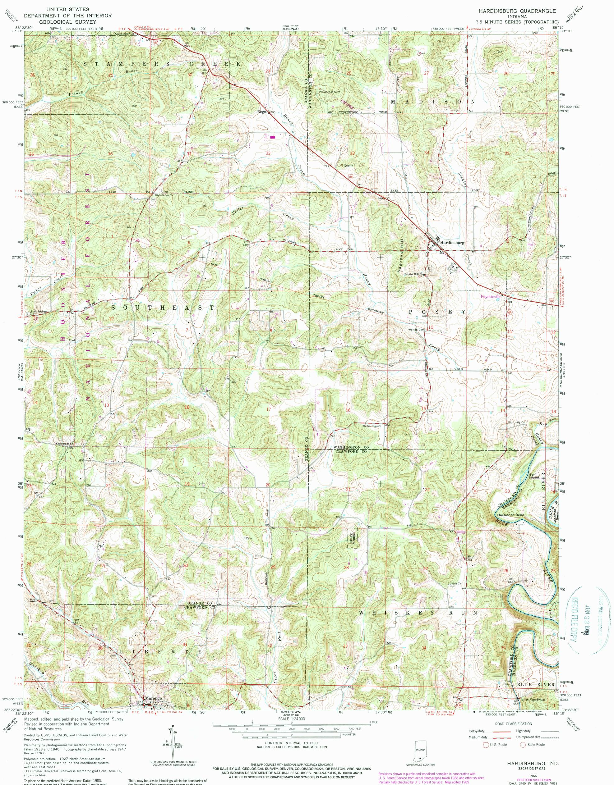
To place on the predicted North American Datum 1983, move the projection lines 3 meters south and 1 meter west as shown by dashed corner ticks
