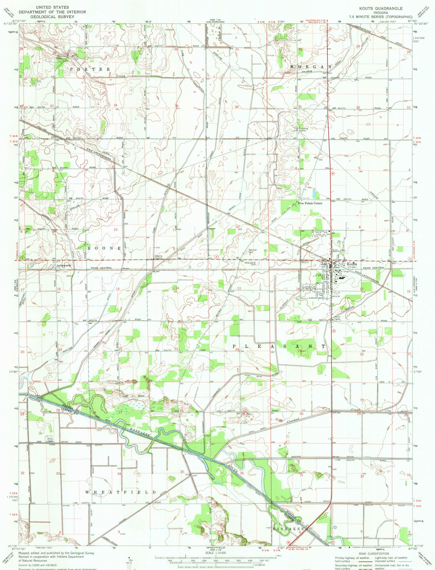
Planimetry by photogrammetric methods from aerial photographs taken 1952. Topography by planetable surveys 1953. Revised from aerial photographs taken 1969. Field checked 1969
