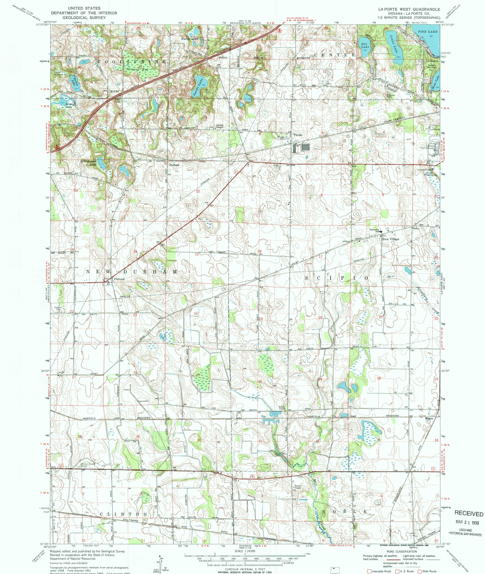
Topography by photogrammetric methods from aerial photographs taken 1958. Field checked 1961 Revised from aerial photographs taken 1969. Field checked 1969
